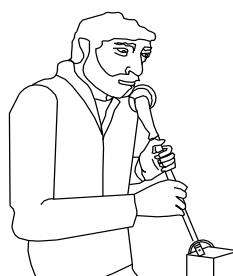
Rest the scraper handle against your shoulder and keep the scraper blade tip in contact with the workpiece.
