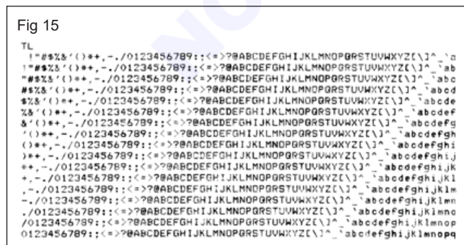
Fig 16 shows a print head test page for identifying defects in print heads
