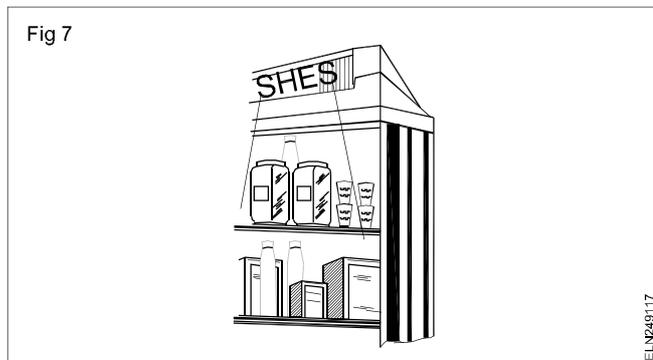
For lighting displays on columns or built-in shelving a metal nosing along the front edge of each shelf effectively conceals small 25 watt tubular lamps as shown in the sketch. Lamps should be spaced not more than 30 cms apart. Lumiline lamps are, of course, equally suitable in many cases.
