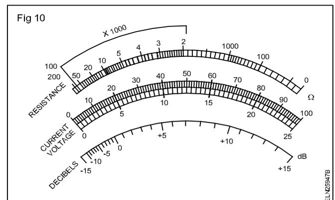
The scale of current and voltage is uniformly graduated.
