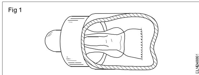
This type of construction results in lower electrode losses. The other details of construction for instant start fluorescent tubes are the same as for preheat fluorescent tubes with the exception that the diameter of the instant start tubes is slightly smaller than that of the pre-heat fluorescent tubes.
