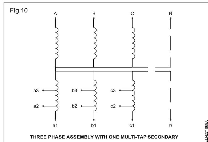
The letters A,B,C denote fully insulated terminals and the letter N denotes a terminal intended to be earthed and the insulation of which is less than that of the other terminals.
