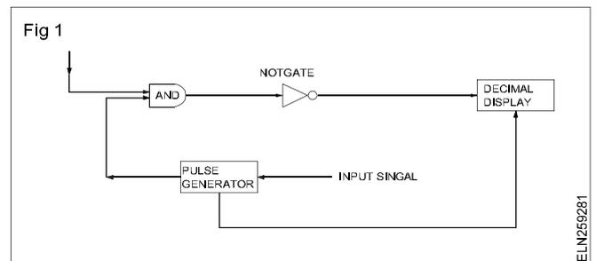
**Input signal:** It is basically the signal of voltage to be measured.
