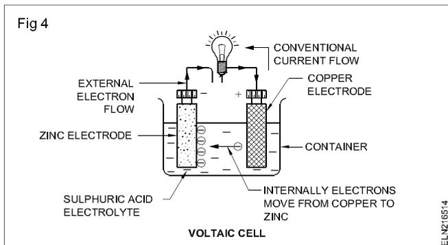
The electric current will flow as long as the chemical action continues. In this type of cell the zinc electrode is eventually consumed as part of the chemical reaction. The voltaic cell is also known as a wet cell because it uses a liquid solution for the electrolyte.
