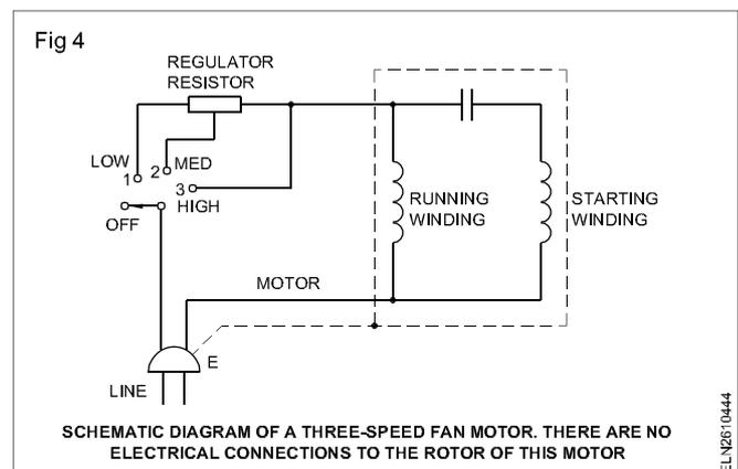
Then, if the fan motor will run only on high or medium speed but not on low speed, the problem is usually in the portion of the series resistor between the medium and low terminals. Or, if the fan motor runs only in the high position, the trouble is in the series resistance between the high and medium terminals. Also check for a dirty switch and a loose contact or wire. Often a dirty switch contact will cause one or more speeds to go dead.
