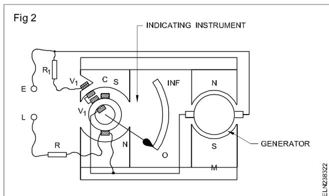
A generator commonly called a magneto is often designed to produce various voltages. The output may be as low as 500 volts or as high as 1 megavolt. The current supplied by the megohmmeter is in the order of 5 to 10 milliamperes. The meter scale is calibrated: kilo-ohms (K  $\Omega$ ) and megohms (M  $\Omega$ ).
