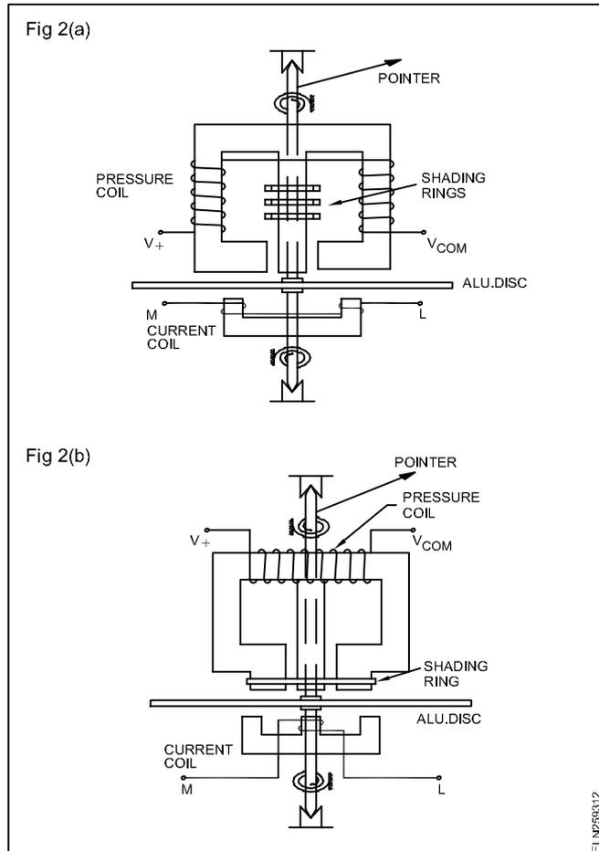
Both the types have one pressure coil magnet and one current coil magnet. The pressure coil carries a current proportional to the voltage whereas the current coil carries the load current.
