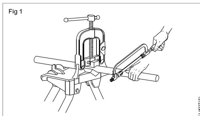
inner edge of the cut. Be sure this ridge is removed and the conduit is smooth before installing a coupling or any fitting, to avoid damage to the insulation of conductors.
