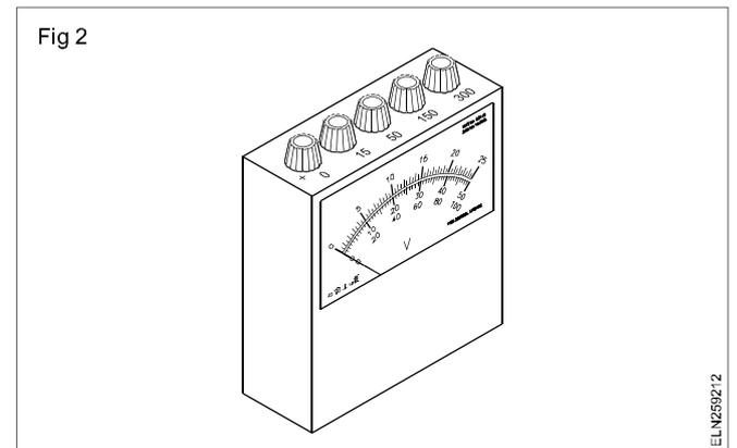
A range selector switch is used in some meters (Fig 3). While reading such meters, care should be taken to keep in mind the position of the range selector switch, and read the scale reading corresponding to that selected range.
