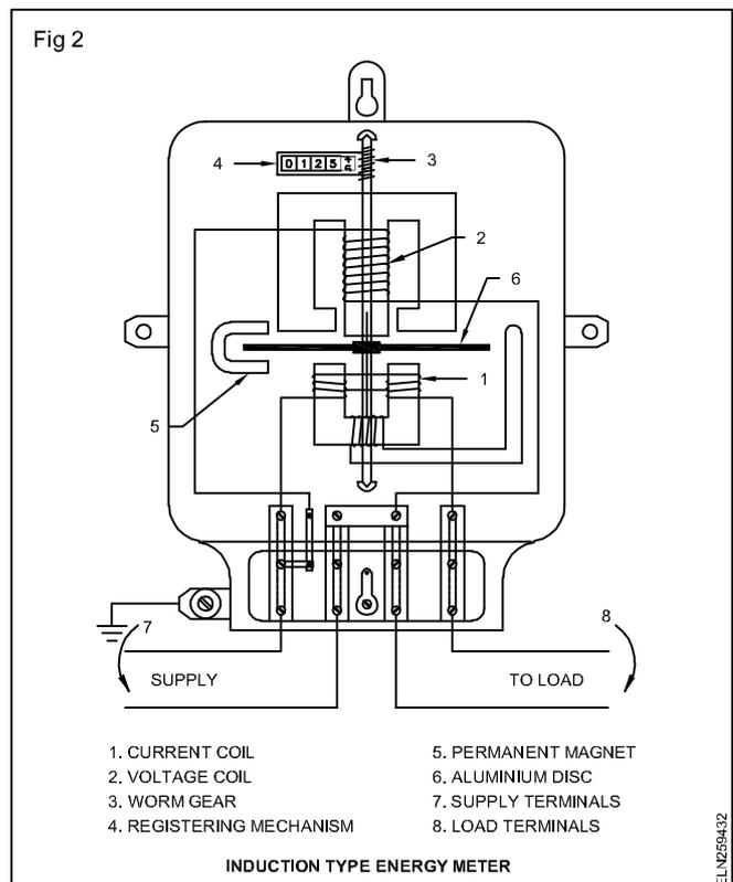
The speed of rotation of the aluminium disc is proportional to the product of the amperes (in the current coils) and the volts (across the potential coil). The total electrical energy that is consumed by the load is proportional to the number of revolutions made by the disc during a given period of time.
