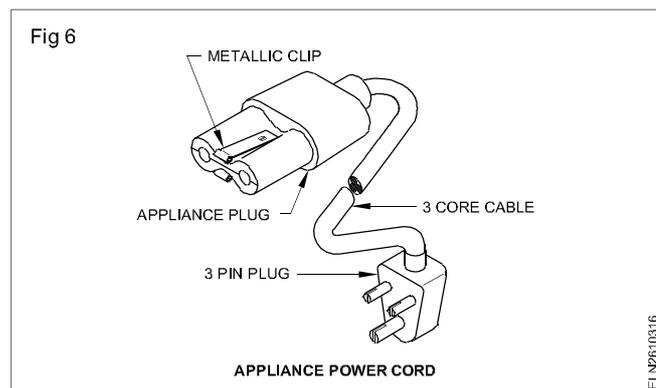
For this the appliance plug has two spring-loaded, metallic clips on either side of it which makes the contact with metallic enclosure of the socket when plugged. As rusting prevents proper contact of these clips with the socket, for safety, these clips and sockets are made of nickel-plated brass. If the spring tension of the clip is lost, it should be replaced. Otherwise earth contact will not be proper.
