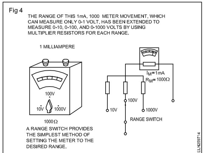
**Sensitivity of voltmeter:** An important characteristic of any voltmeter is its impedance or ohms per volt (ohms/volt) rating. Ohms/volt rating is the voltmeter sensitivity. The ohms/volt rating is defined as the resistance required ( $R_M + R_{MULT}$ ) for full scale deflection. For example, the 1mA 1000 ohms meter movement indicates 1 volt at full scale deflection. Therefore its 'ohm/volt' rating is 1000/1 or 1000 ohms/volt (Fig 3) ohms/volt =  $E_{MAX} / I_M$ .
