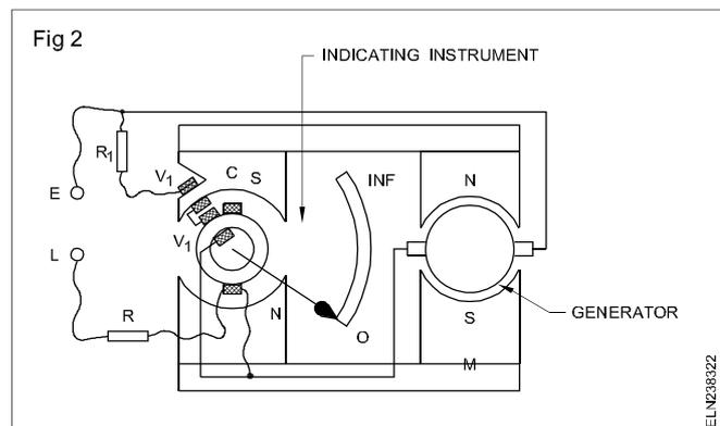
A generator commonly called a magneto is often designed to produce various voltages. The output may be as low as 500 volts or as high as 1 megavolt. The current supplied by the megohmmeter is in the order of 5 to 10 milliamperes. The meter scale is calibrated: kilo-ohms (KΩ) and megohms (MΩ).
