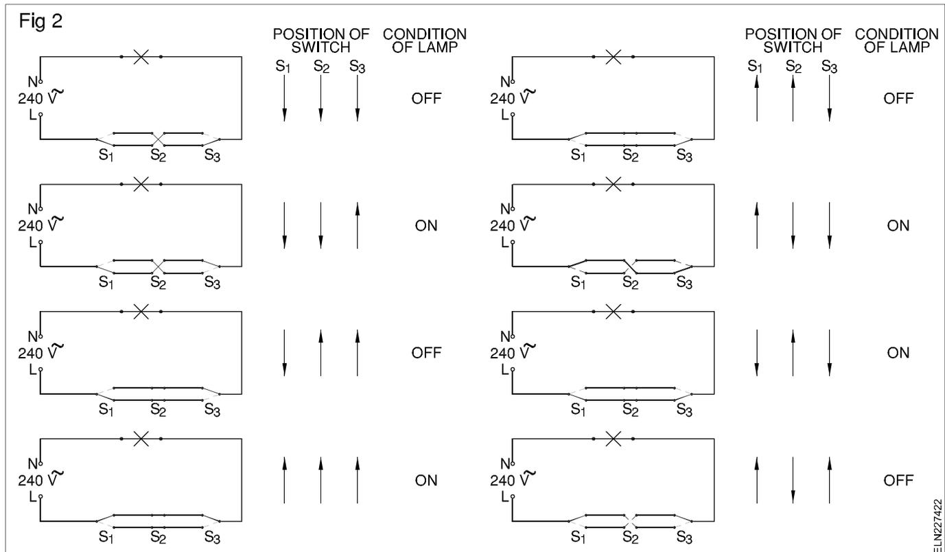
To control a lamp from three locations, three intermediate switches instead of a two two-way switches can also be used. (But, in practice, they are not used since it is very expensive).
