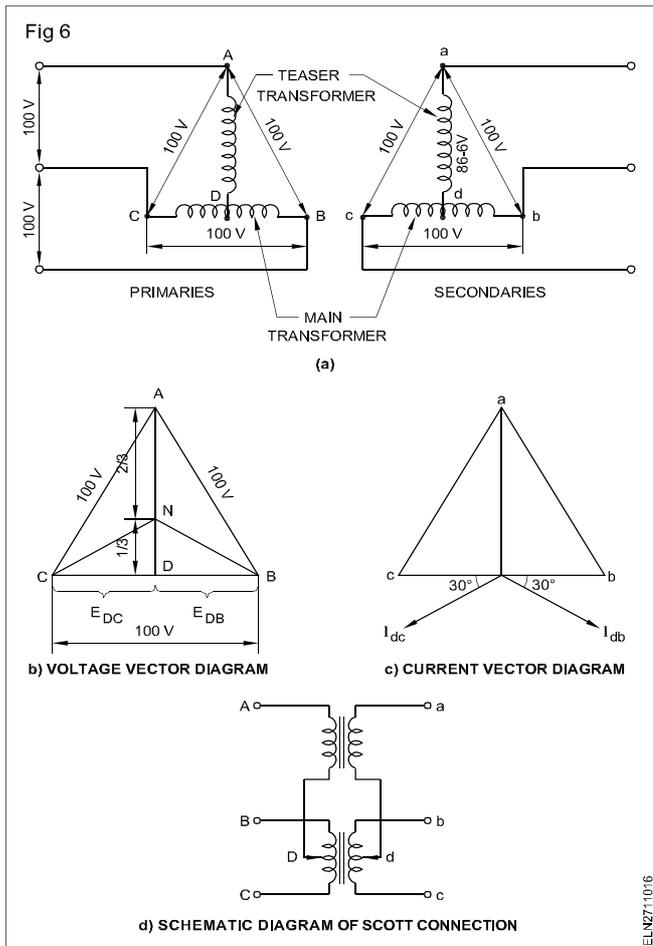
By analysing the vector diagram Fig6b, it is found that voltage  $E_{DC}$  and  $E_{DB}$  are each 50V and differ in phase by  $180^\circ$  because both the coils DB and DC are in the same magnetic circuit and are connected in opposition. Fig 1d shows the schematic connection diagram.
