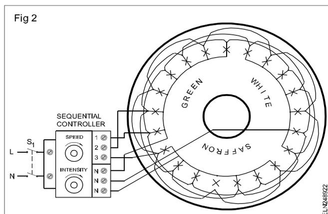
The circumference of the cans or the drums are so cut that the brushes will make contact only during the fixed portion of the revolution, thus completing the circuit. We can make three independent circuits by the 3-point sign flashers which are switched 'ON' and 'OFF' successively.
