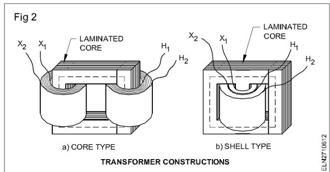
Normally, this is not a desirable design. Its disadvantage is the large leakage fluxes associated with it. The large leakage fluxes cause poor voltage regulation. Therefore, to ensure that most of the flux set by the primary will link the secondary, the construction Fig 2b is employed. This is called shell type construction.
