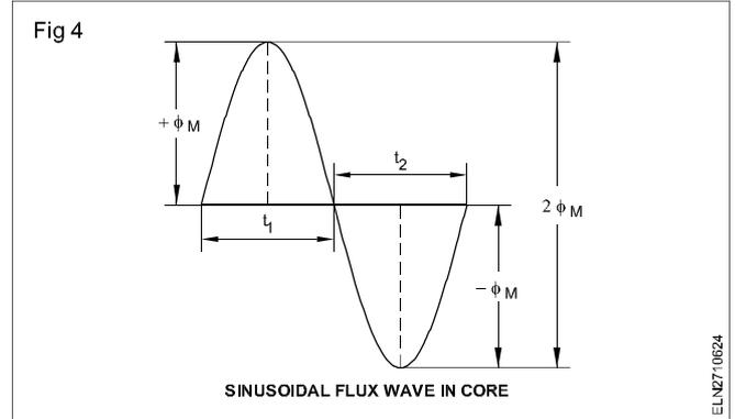
$$E_{avg} = \text{turns} \times \frac{\text{change in flux in a given time}}{\text{given time}} \dots(1)$$
