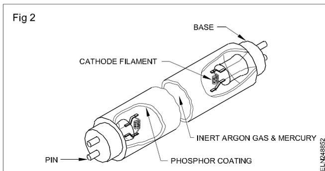
The inner surface of the tube is coated with a fluorescent powder or phosphor. This phosphor emits light when exposed to ultra-violet rays. Cathodes or electrodes are
