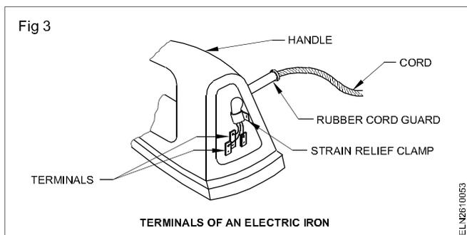
**Handles:** Handles are made of wood or plastic. In modern irons, plastic handles are made in large units combining the handle and brackets in a single unit mounted directly on the cover. Sometimes handles are split to provide access to the terminal covering and an entrance for the cord. When disassembling an iron for repair, the handle and its part are usually the first to be disassembled.
