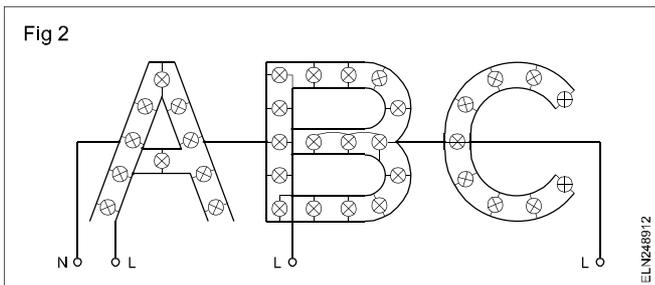
Mark the lamp position on the layout, connect all the lamps in parallel of letters A, B and C as shown in Fig 2, and then test the lamps for each letter by effecting supply. The neutral is run to all the lamps commonly.
