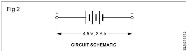
V Battery = V per cell x No.of cells
