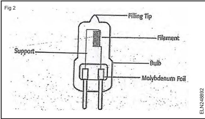
To maintain this regenerative cycle, it is necessary that the wall temperature is maintained high to 2500°C. The lamp envelope is therefore made of quartz due to which it is possible to miniaturise, as filling gas can now be filled at high gas pressure.
