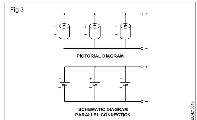
Identical cells are connected in parallel to obtain a higher output current or ampere-hour rating. With this connection of cells, the output ampere hour rating is equal to the sum of the ampere hour ratings of all the cells. However, the output voltage remains the same as the voltage of a single cell.
