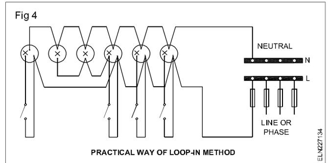
**Loop-in method by 3-plate ceiling rose:** We can also use 3-plate ceiling roses (Fig 4). Considerable cable length could be saved by using the third terminal of the ceiling rose as a looping-in terminal for the switch drop, so that two cables only are required from the ceiling rose to the switch.
