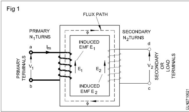
The applied voltage causes a small current to flow in the primary winding. This no-load current is meant to build up a counter-electromotive force equal and opposite to the applied voltage.
