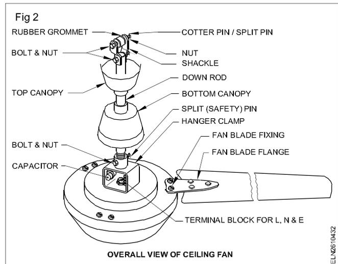
The fan blades are made from aluminium sheet. The size of the fan blades will depend on the area of the room, usage and appearance. The performance of the fan depends on the number of blades and their pitch angle, say 10 to 15°. Ceiling fans are available with three or four blades. The size of the fan is generally determined by its **sweep**. The following sweeps are available, 900 mm, 1050 mm, 1200 mm and 1400 mm.
