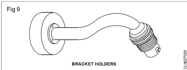
These are fixed on the bracket by the internal threading of the cap.
