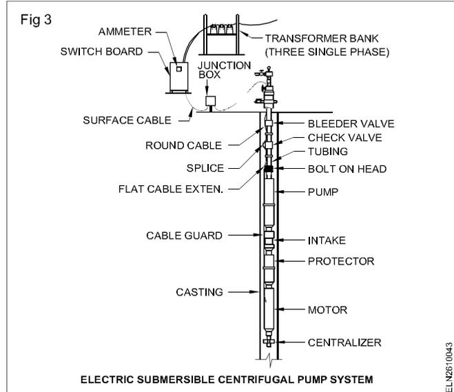
**Submersible pumps** : This pump also comes under the category of centrifugal pumps and is found in use at places where water is found in great depth.
