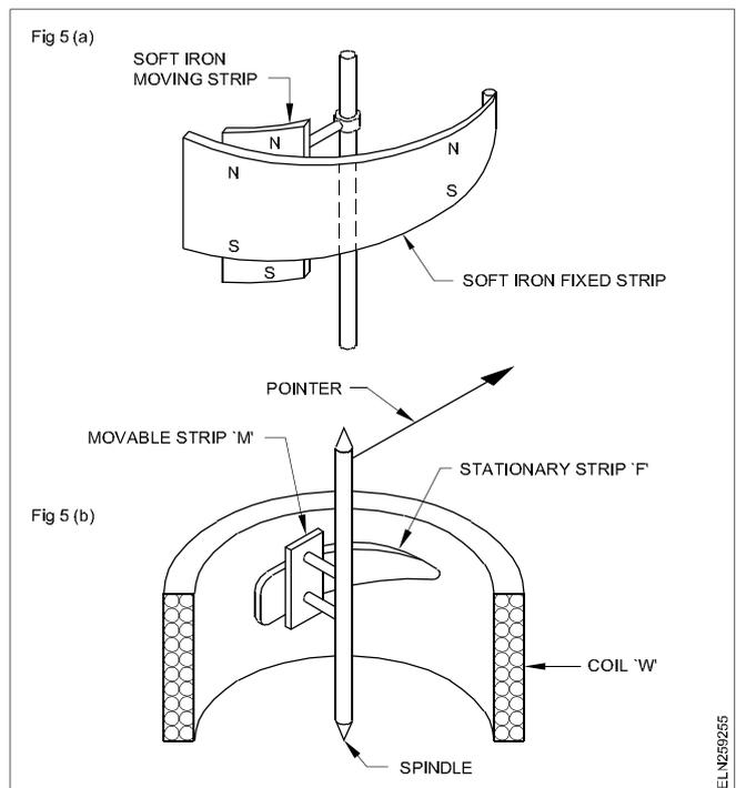
The torque, which is proportional to the square of the current, is proportionally reduced by the narrow portion of the fixed iron, resulting in more or less even torque and thereby uniform scale.
