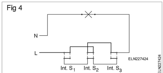
The schematic diagram (Fig 5) is for controlling one lamp from five locations using two two-way switches and three intermediate switches is given below.
