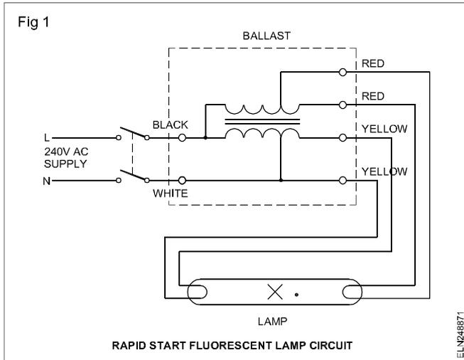
Since the cathodes are already heated, the amount of voltage required to cause the lamp to fluoresce is smaller than the voltage required for the instant start lamp. As a result, the rapid start system is very efficient particularly because of the small amount of loss in the ballast.
