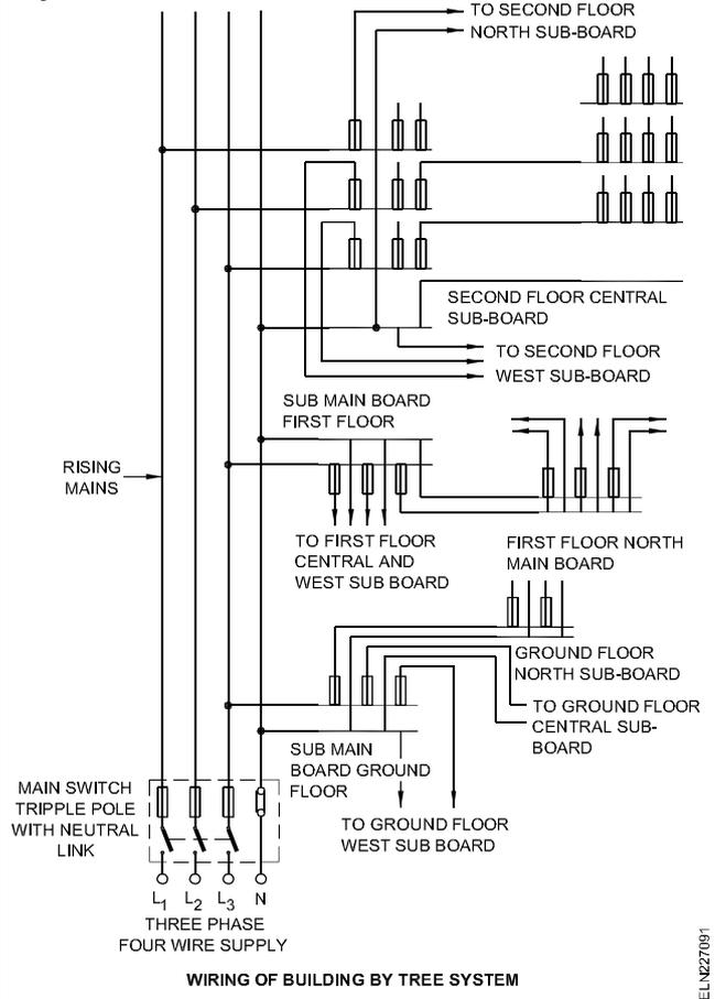
At each floor the running main is connected to the sub-main board through proper cable terminations. If there are more than one flat in each floor the individual main switches for the flat get their supply from the sub-main board through a distribution network which may include an energy meter for each flat.
