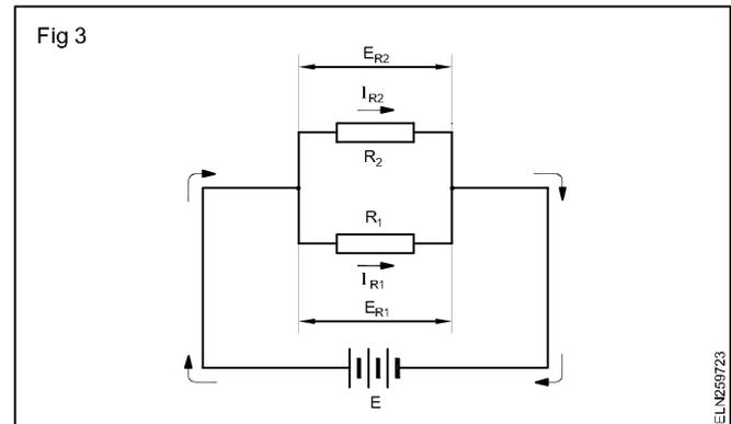
Since the same voltage appears across  $R_1$  and  $R_2$  then  $E_{R1} = E_{R2}$ . From this we derive  $I_{R1} R_1 = I_{R2} R_2$ . This equation can be used to calculate the shunt needed for a particular current measurement.
