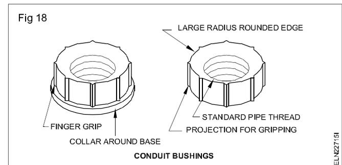
second purpose is to give a proper grip mechanically and make the conduit electrically continuous in the installation.
