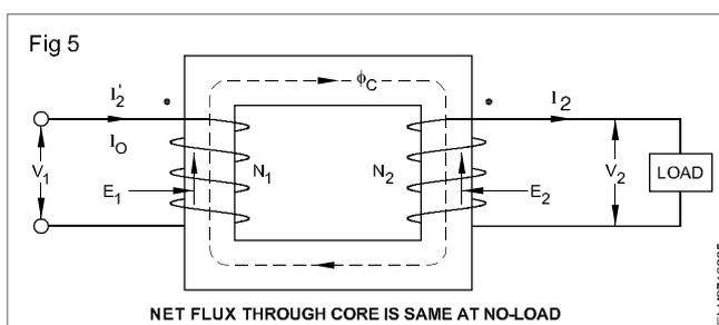
When the transformer is in no-load, the primary winding has two currents  $I_o$  and  $I_2'$ . The total primary current  $I_1$  is the vector of  $I_o$  and  $I_2'$ . The elementary vector diagram of the transformer with load ( Fig 6)
