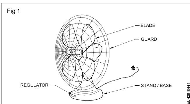
The table fan motor is mostly of a capacitor start or split phase, single phase induction type.
