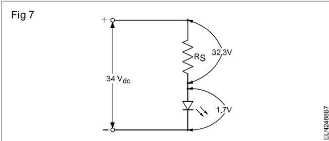
For the LED to give reasonably good light, the current through the LED has to be 20 mA, as indicated in the specifications sheet. So, the value of  $R_s$  must be,
