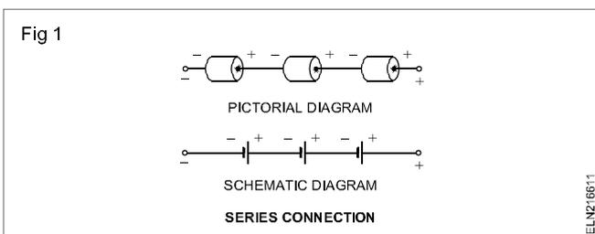
Identical cells are connected in series to obtain a higher voltage than is available from a single cell. With this connection of cells, the output voltage is equal to the sum of the voltages of all the cells. However, the ampere hour (AH) rating remains equal to that of a single cell.
