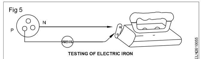
Connect two ends of the testing leads to the terminals of the iron. If the lamp gives dim light, it means that the element is in working order. If the lamp does not light up, there is breakage in the element or disconnection of the strip from the terminal.
