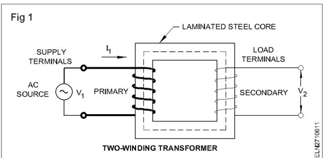
Laminated steel core transformers are used in power applications. Fig 1, the current flowing in the coil connected to the AC source is called the primary winding or simply primary. The primary is the input to a transformer. It sets up the flux in the core, which varies periodically both in
