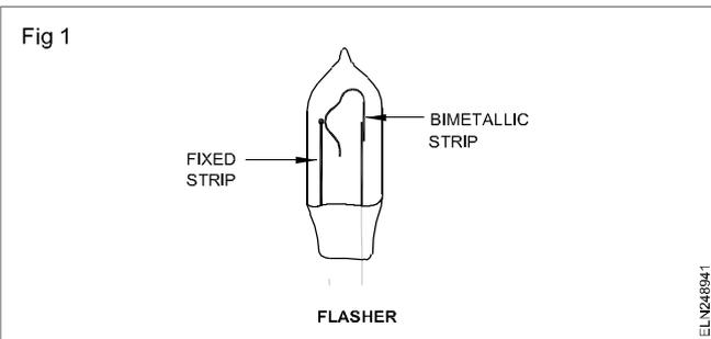
When the row of lamps is connected across the supply and switched ON, the bimetal strip gets heated up, this breaks the contacts and disconnects supply to the other lamps, making the lamps OFF.
