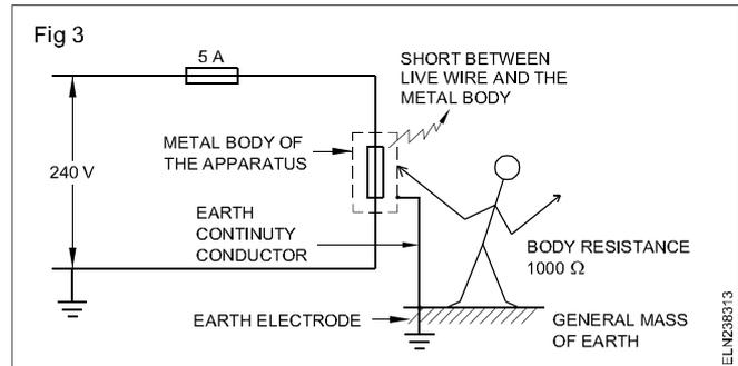
Assuming that the sum of the resistance of the main cable, metal body, earth continuity conductor and the general mass of earth is to the tune of 10 ohms
