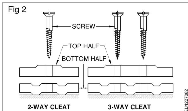
Initially the bottom and top cleats are fixed on the wall loosely according to the layout. Then the cable is drawn through the cleat grooves, and it is tensioned by pulling and the cleats are tightened by the screw.
