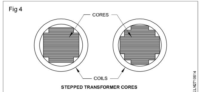
In practice, the primary and secondary windings of a transformer have two or more coils per leg. They may be arranged in series or parallel. The laminations are pressed together by clamping in such a way as to prevent any fluttering or shifting.
