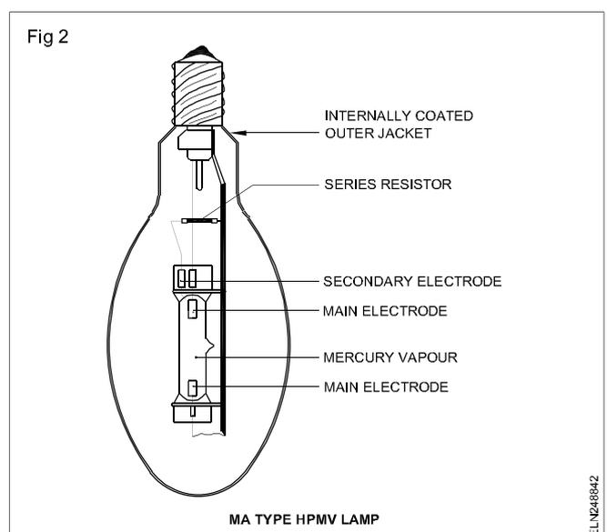
This lamp, once switched off, will not restart again until the pressure developed inside the tube falls back. It takes about 7 minutes to start again. There is no harm in keeping the switch on. The lamp should always be hung vertically, otherwise the inner tube will be damaged.
