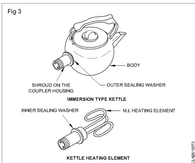
New elements can be fitted to most types of kettles without difficulty.
