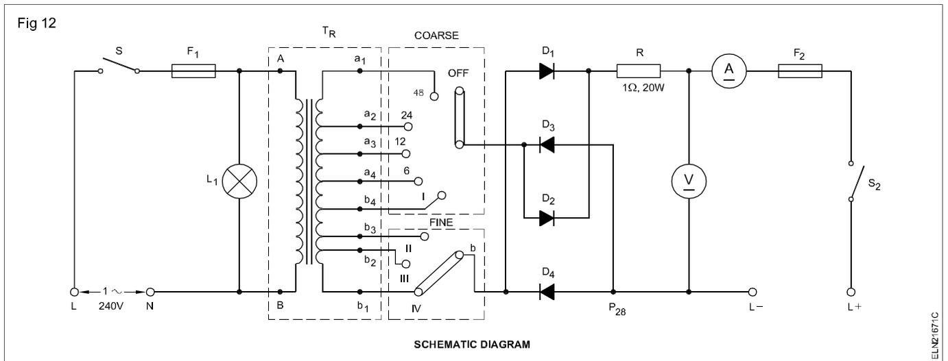
Further the charging current could be varied through one or more selector switches where tappings are made for lower voltage ranges. A full wave rectifier with four power diodes are used to form the bridge.
