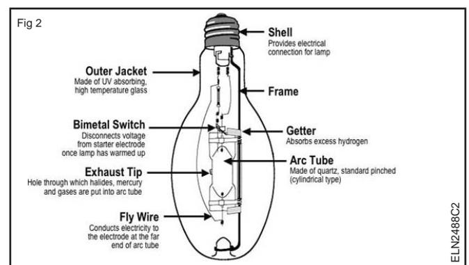
Light is generated by creating an arc between the two electrodes located inside the inner arc tube. The inner arc tube is typically made of quartz, and this is a very harsh environment, with high temperatures approaching 1000°C and pressure of 3 or 4 atmospheres.
