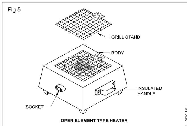
**Heater socket:** This is used for plugging the power supply appliance plug. The socket (Fig 6) has two male terminals, one for the phase, and the other for the neutral. However, for safety, the heater body should be connected to the general mass of earth through the earth continuity conductor.
