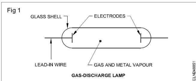
A glass shell with two electrodes apart is connected through lead in wires to the voltage source. The space within the shell is filled with low pressure vapour. When the voltage applied to the electrodes is increased to a certain value, the gas inside gets ionised and starts conducting.
