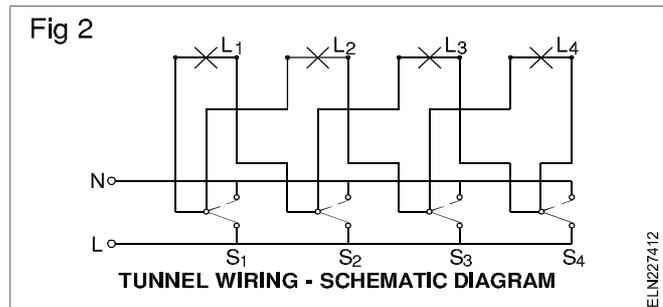
In tunnel wiring a person walking along the tunnel can successively light behind two lamps ahead and put off a lamp behind with one switch.
