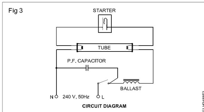
Function of the various parts in a fluorescent light circuit
