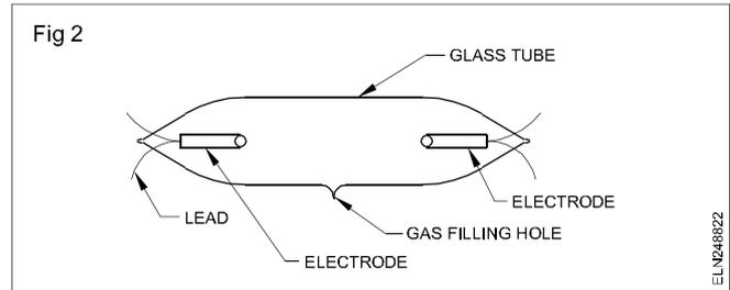
The length of the tube varies from 1 metre to 5 metres, and the diameter varies from 10 mm to 20 mm. The tubes are joined with electrodes which are operated at high voltage. The electrodes are connected with nickel wires for more length or to different letters. (Fig 3)
