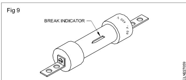
Normally a silver alloy is used as the fusing element and when it melts due to the excessive current, it combines with the surrounded sand/powder, and forms small globules without making an arc, spark or gas. HRC fuses can open a short-circuited circuit within 0.013 second. It has an indicator to show the fuse has blown. The rupturing capacity of the fuse could be calculated from the following formula.
