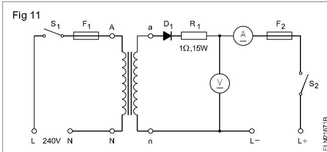
This type of circuit is protected only through fuses and needs constant attention during the entire period of battery charging. As the output voltage is fixed, only particular rated voltage batteries or a combination of them could be charged.
