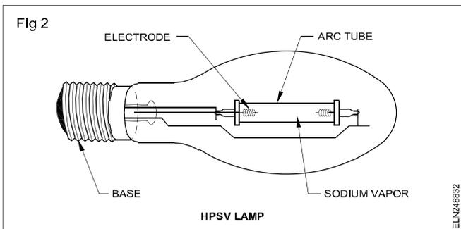
This discharge tube is made of sintered aluminium ceramic discharge arc tube which is resistant to the hot ionised Sodium Vapour up to a temperature of about 1600°C which transmits over 90% of visible radiation.
