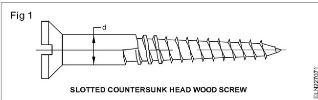
In electrical wiring for fixing wooden blocks, boards, battens and electrical accessories, countersunk holes should be used. The screw shall be driven until the head is flush with the work or slightly below surface.
