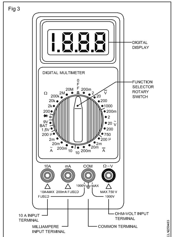
**DMM functions:** The basic functions found on most DMMs are the same as those on analogue multimeters. That is it can measure:-
