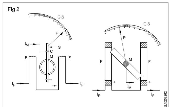
**Working:** As shown in Fig 3, let the current passing through the fixed coils be  $I_F$ , and the current passing through the moving coil be  $I_M$ . The field strength will be proportional to the current  $I_F$ .
