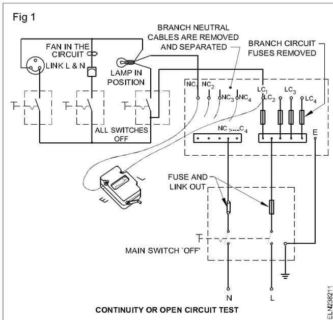
By switching the switches ON and OFF one by one, the Megger should show zero reading and infinity alternatively. The two-way switches may have to be operated alternatively to ensure the correct test results.
