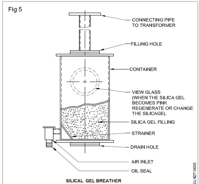
The oil seal at the bottom of the breather absorbs the dust particles that are present in the air entering the conservator.
