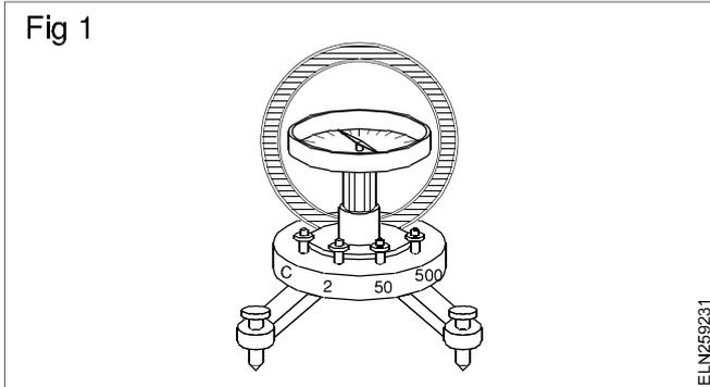
**Secondary instruments:** In these instruments the value of electrical quantity (voltage, current, power, etc.) to be measured can be determined from the deflection of the instruments on the calibrated dial. These instruments should be calibrated in comparison with either an absolute instrument or with one which has already been calibrated. All the instruments used commercially are secondary instruments.
