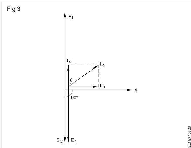
**Theory of No-load Operation:** With the secondary winding open-circuited, the no-load current  $I_o$  flows in the primary winding. This no-load current has two functions:
