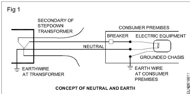
Earth point is the point connected to the ground, i.e. earthed locally at the consumer premises while Neutral point is the star point of the secondary stepdown transformer feeding the consumer premises.
