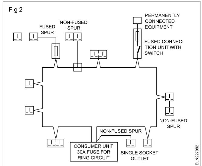
As per IEE regulations one ring circuit has to be there for every 100 sq metres of the floor area or part thereof. The number of power plugs fed from branch lines (spurs) should not exceed two and the total current should not exceed 30 amps. Protection for individual power plug can be provided by having built-in-fuses with the individual power plugs or by having MCB type switch and socket arrangement.
