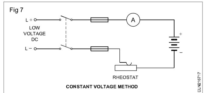
**Use:** For charging batteries of constant voltage rating.
