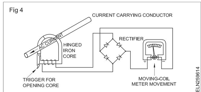
The core is so designed that there is only one break in the magnetic path. The hinge and the opening both fit tightly when the instrument closes around the conductor. The tight fit of the instrument ensures minimum variation in the response of the magnetic circuit.
