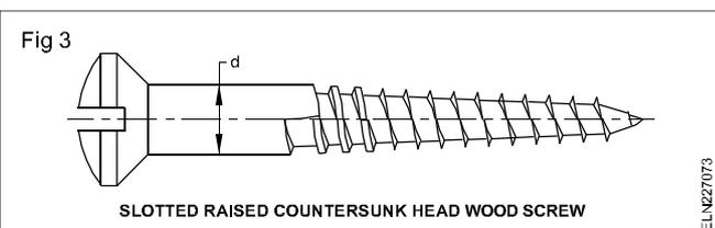
Of the three types of screws listed above, countersunk (flat head) screws are commonly used for electrical wiring installations.
