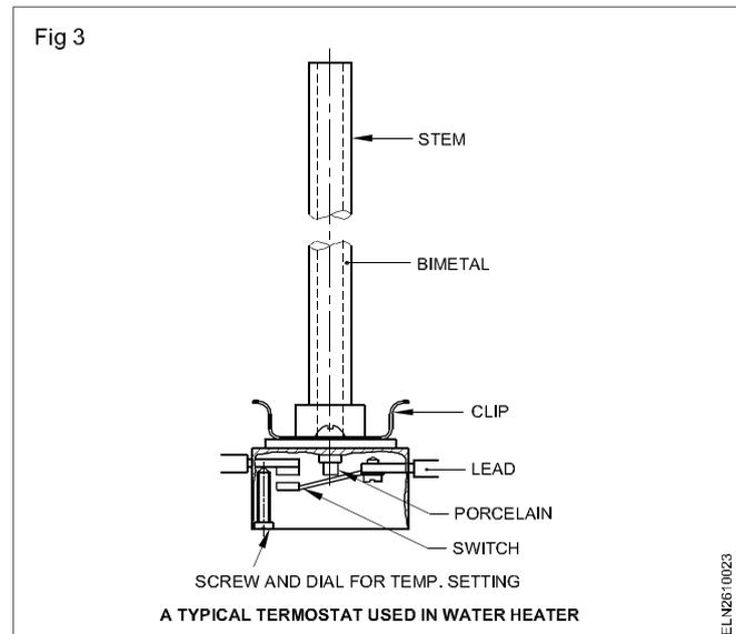
Thermostats are available in sizes of 8 mm diameter with a length of 175 mm, 275mm or 450 mm depending on the height of the geyser. Thermostats are fixed in a tube and are connected in series with the heating element.
