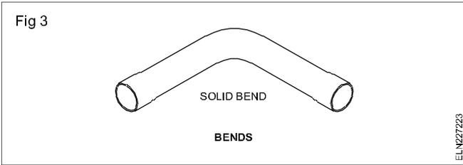
A bend gives a diversion of 90°C in the turn of a conduit, and a normal bend shall be a large sweep. Inspection type bends are used to assist in the inspection at the corners and for drawing cables.
