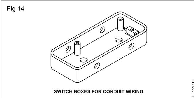
The ceiling, wall and switch boxes are normally provided with knock-out openings which can be removed when required by using punches or chisels with a stroke from a hammer. In some cases the knock-out openings could be made by the pry out-method with a screwdriver (Fig 15).
