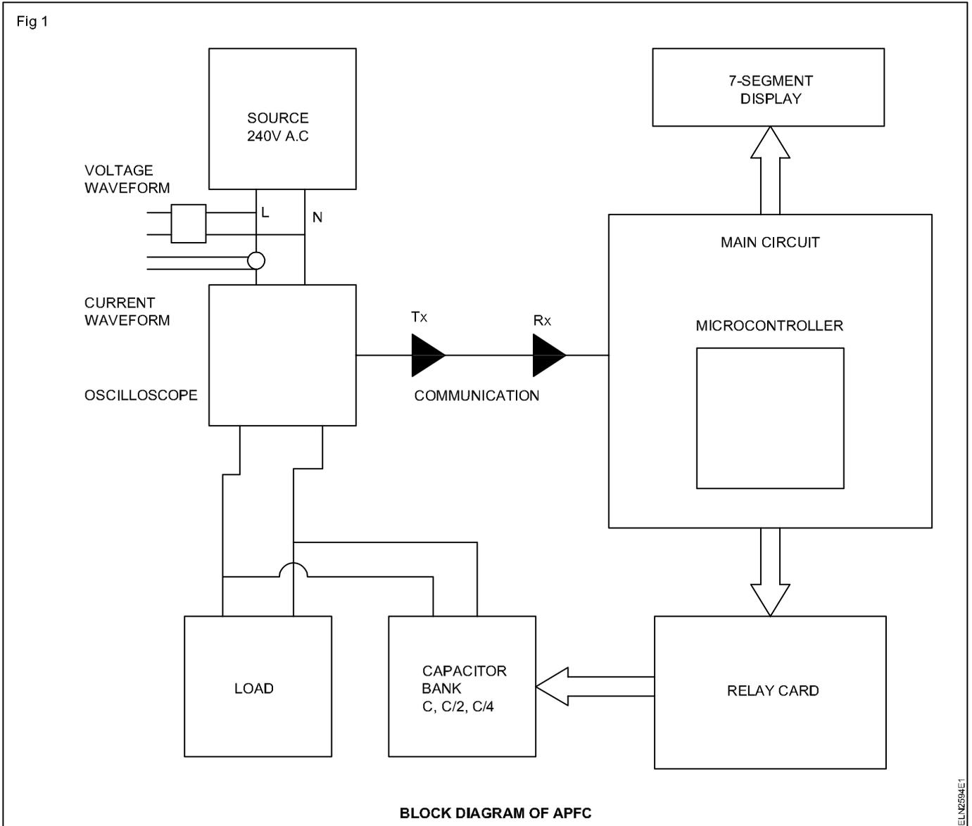
The power factor meter is used to calculate the present power factor of the system. The power factor is corrected using the true power technique. The power factor value so obtained is communicated to the microcontroller via the pins TX and RX.
