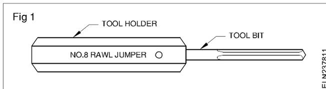
The tool bit is fluted to allow maximum debris clearance and ensure fast penetration. The shank of the tool bit is tapered to fit into the tool holder.
