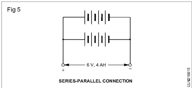
The number of cells that must be connected in series to have voltage rating is calculated first and then the number of parallel rows of series connected cells is calculated for required ampere-hour rating.
