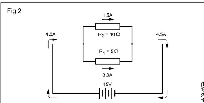
Current flow divides between two resistors parallel in a ratio inversely proportional to their resistance.
