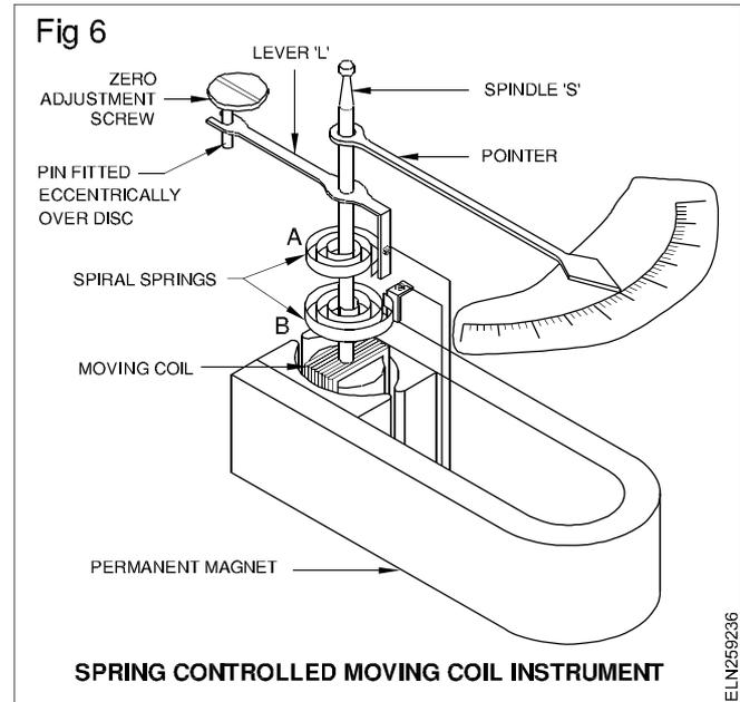
winds up while the other unwinds, and the controlling force is due to the combined torsions of the springs.
