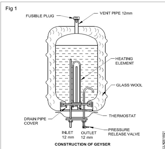
The outer casing is made of mild steel sheet. The inner tank is made of heavy gauge copper which is tinned to prevent corrosion. The space between the outer casing and the inner tank is filled with glass wool as heat insulation to avoid excess heat losses. Heating elements, thermostat, inlet and outlet pipes are fitted to the tank.
