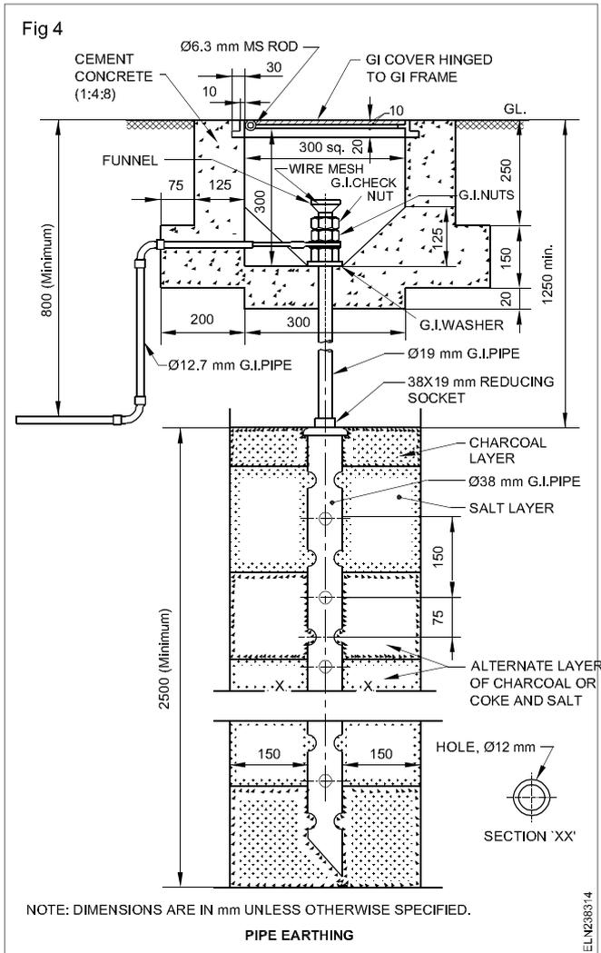
Pipe electrodes shall not be smaller than 38 mm internal diameter, if made of galvanised iron or steel, and 100 mm internal diameter if made of cast iron.
