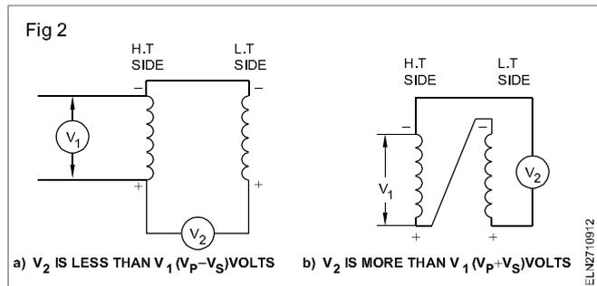
If in transformer has similar ends in one side (Fig 3a) the polarity marking is said to be subtractive polarity marking on the other hand if the opposite ends are in one side ( Fig 3b) the polarity marking is called as additive polarity marking.
