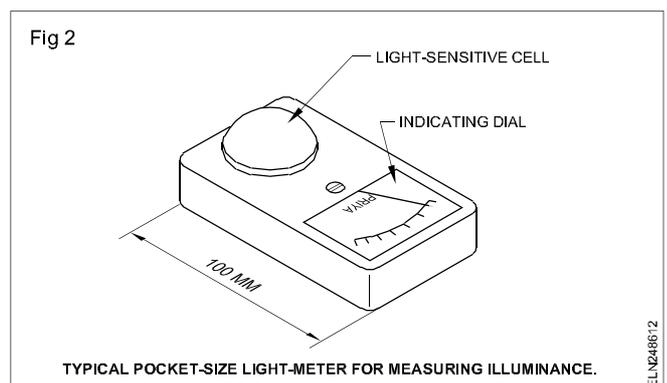
Measured brightness is termed 'luminance', and it should not be confused with 'illuminance'. Luminance is the lumens emitted by a luminous surface of one square metre.
