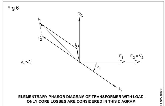
**Leakage fluxes:** When a current flows in the secondary winding, the resulting mmf ( $N_2 I_2$ ) creates a separate flux, apart from the flux  $f_c$  produced by  $I_o$ , which links the secondary winding only. This flux does not link with the primary winding and is therefore not a mutual flux.
