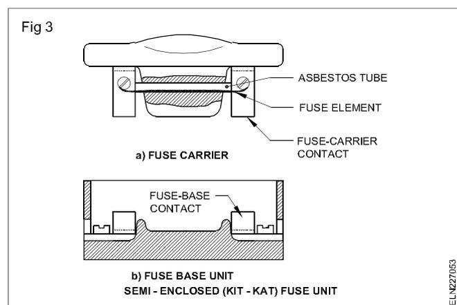
The fuse elements used in this type are tinned copper wire, lead and tin alloy or aluminium wire (Table 1).
