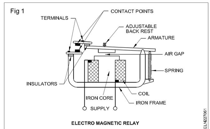
**Current sensing relay:** A current sensing relay functions whenever the current in the coil reaches an upper limit. The difference between the current specified for pick up (must operate) and non-pick up (must not operate) is usually closely controlled. The difference in current may also be closely controlled for drop out (must release) and non-drop out (must not release).
