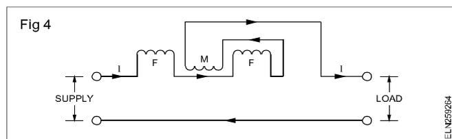
As the moving coil is made by winding small gauge (thin) wire, the above connection is unsuitable for measuring heavy currents.
