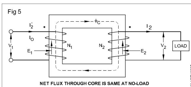
When the transformer is in no-load, the primary winding has two currents  $I_0$  and  $I_2'$ . The total primary current  $I_1$  is the vector of  $I_0$  and  $I_2'$ . The elementary vector diagram of the transformer with load ( Fig 6)
