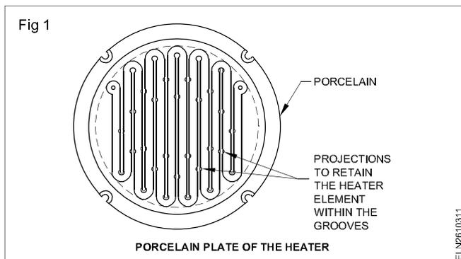
Porcelain withstands high temperature and remains as a good insulator even at high temperatures, say 1300°C. The coiled Nichrome heating element is housed in the grooves. The grooves are designed with projections at various places (Fig 1). The projections prevent the heating element from coming out of the grooves.
