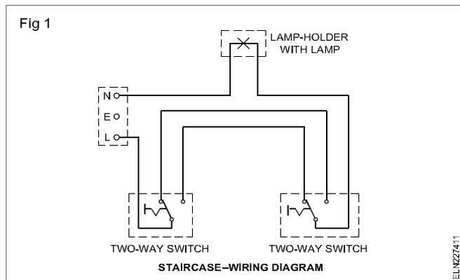
In the case of godown wiring we have seen that as you move inside the godown, you can switch on a lamp ahead of you while the light behind you is put off. The same process in the reverse order takes place while moving out of the godown.
