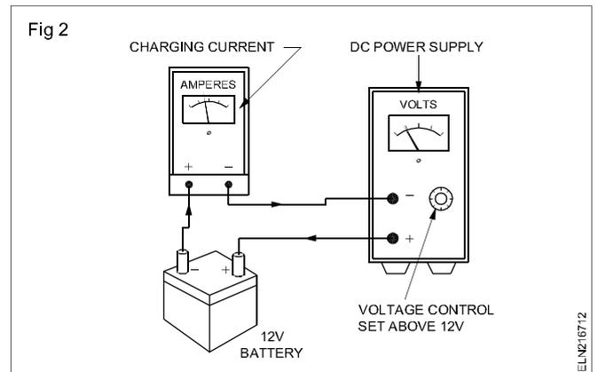
Before charging the battery or cell the following points are to be observed to ascertain the condition of the battery.
