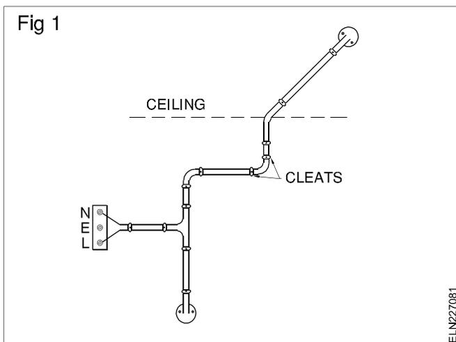
Cleat wiring is recommended only for temporary installations. These cleats are made in pairs having bottom and top halves (Fig 2). Bottom half is grooved to receive the wire and the top half is for cable grip.
