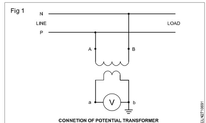
If the primary turns are four, the secondary turns are two and the primary is connected to a voltage source of magnitude 220 volts, the secondary voltage will be 110 volts according to the transformation ratio.
