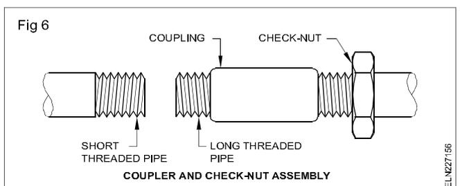
First the check-nut and then the coupler should be screwed inside the long threaded conduit. Then the short threaded conduit is butted with the long threaded conduit and the coupler is screwed on the short threaded conduit tightly.
