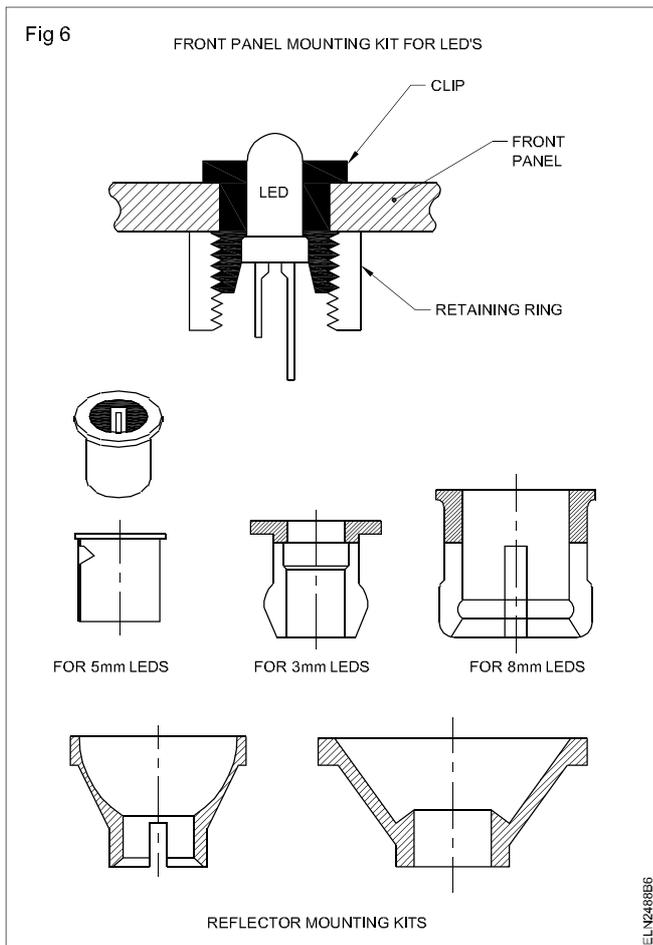
Special mounting kits Fig 6, are available for fixing the LEDs on to the printed circuit boards and monitoring panels. These kits not only extend the life of the LED by way of protecting it from mechanical stress but also make the output of the LED clearly visible.
