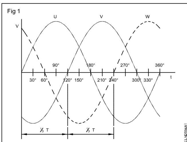
**Importance of correct phase sequence:** Correct phase sequence is important in the construction and connection of various three-phase systems. For example, correct phase sequence is important when the outputs of three-phase alternators must be paralleled into a common
