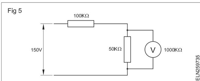
The total resistance of the circuit will be 147.6k ohm (Fig 6).
