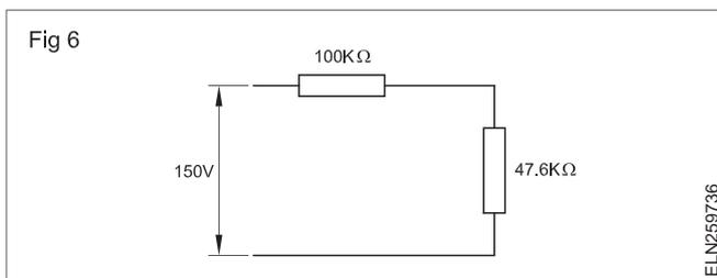
$$V_2 = \frac{47.6k \text{ ohm}}{147.6k \text{ ohm}} \times 150V = 48.36V$$
