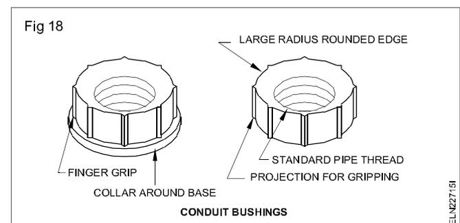
second purpose is to give a proper grip mechanically and make the conduit electrically continuous in the installation.
