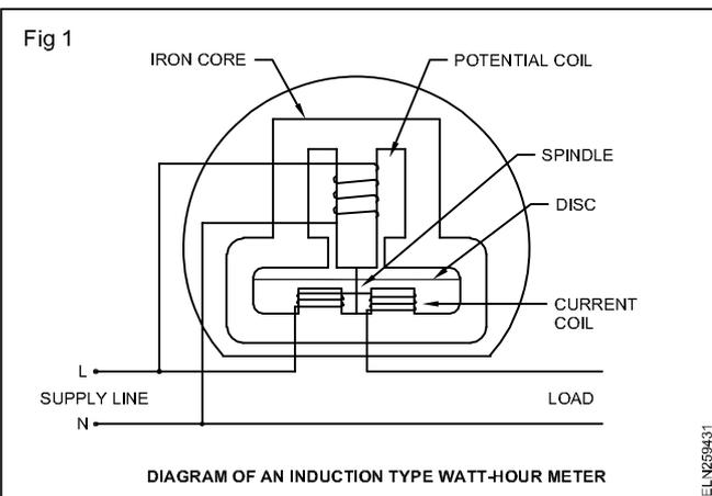
The watt-hour meter must take both power and time into consideration. The instantaneous speed is proportional to the power passing through it.
