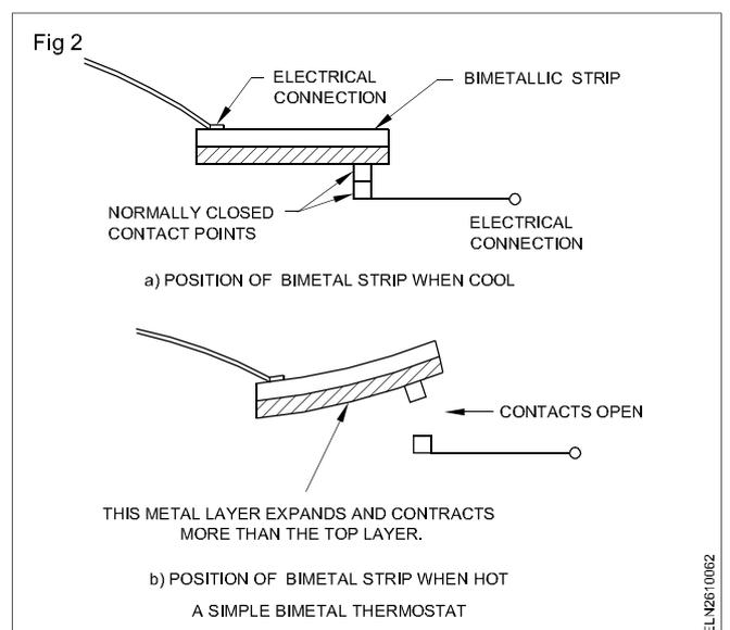
In the thermostat there is a bimetal strip made of two strips of metal with different expansion rates welded together. The metal strip expands when heated and contracts when cooled. One metal in the bimetal strip has a high rate of expansion when heated, and the other has a low rate.
