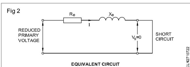
The test is performed on the high voltage side because it is convenient to apply a small percentage of the rated voltage. In the case of a 3300V/240V transformer, it is easier and more accurate to deal with 5% of 3300V than with 5% of 240V.
