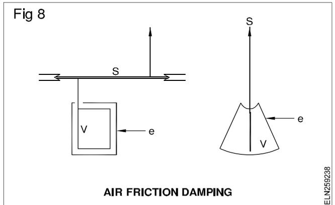
Alternatively, the vane in the form of a piston could be arranged to move inside an air chamber (cylinder) as shown in Fig 9. In the above two cases, the air inside the air chamber opposes the movement of the vane/piston, and, thereby, the damping force is created.
