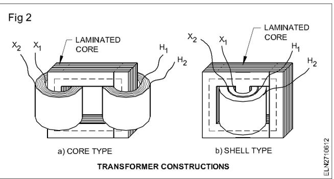
Normally, this is not a desirable design. Its disadvantage is the large leakage fluxes associated with it. The large leakage fluxes cause poor voltage regulation. Therefore, to ensure that most of the flux set by the primary will link the secondary, the construction Fig 2b is employed. This is called shell type construction.
