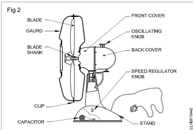
The blades are fabricated out of aluminium for light weight. Modern table fans have moulded blades of plastic material. The sweep of the blade varies from 100mm to 400mm. The number of blades varies from two to six. The speed of the fan is limited to 1000 r.p.m.
