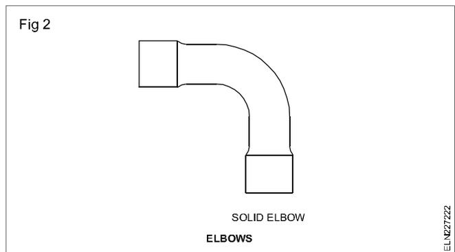
The axis of any elbow shall be a quadrant of a circle plus a straight portion of each end. Elbows are used at sharp ends of nearby walls or roof and wall.
