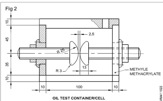
The cell shall have an effective volume between 300 to 500 ml. It should be preferably closed. Section view of container. (Fig 3)
