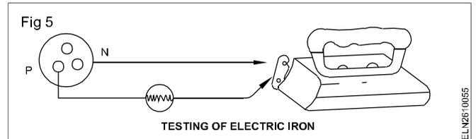
Connect two ends of the testing leads to the terminals of the iron. If the lamp gives dim light, it means that the element is in working order. If the lamp does not light up, there is breakage in the element or disconnection of the strip from the terminal.
