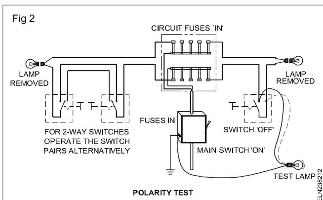
Lighting of the test lamp indicates that the phase or live cable is controlled by the switch.
