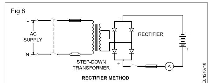
**Trickle charge:** When the battery is charged at a very low rate, that is 2 to 3% of the normal rate for a long period, it is said to be a trickle charge.
