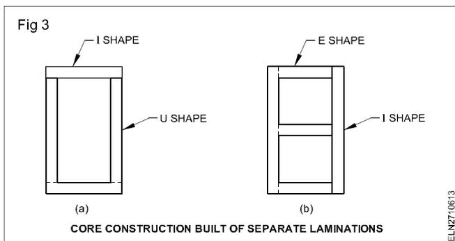
**Core construction :** As a rule, the number of butt joints is to be limited. The joints are tightly made and laminations interleaved so as to minimize the reluctance of the magnetic circuit. The stacking of laminations to the required core cross-section results in the core legs of square or rectangular cross-section. This permits coils to
