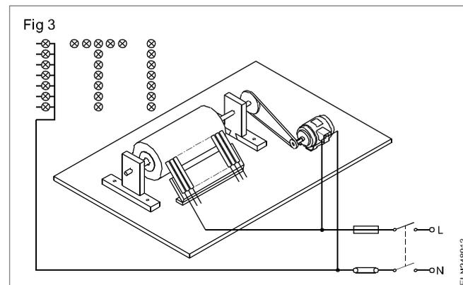
The length of the drum is determined by the number of finger-strips, and the diameter of the drum depends on the number of circuits to be incorporated. The speed of the drum must be as low as possible which is obtained by using two pulleys of different sizes to create a high ratio. (Fig 3) The drum-plates are usually made of brass/copper, and are nailed. The contact strips are fixed by screws or wire nails. (Fig 4)
