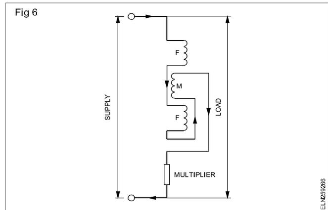
**Dynamometer used as a Wattmeter:** The dynamometer is commonly used as a wattmeter to measure power in both AC and DC circuits and will have uniform scale.
