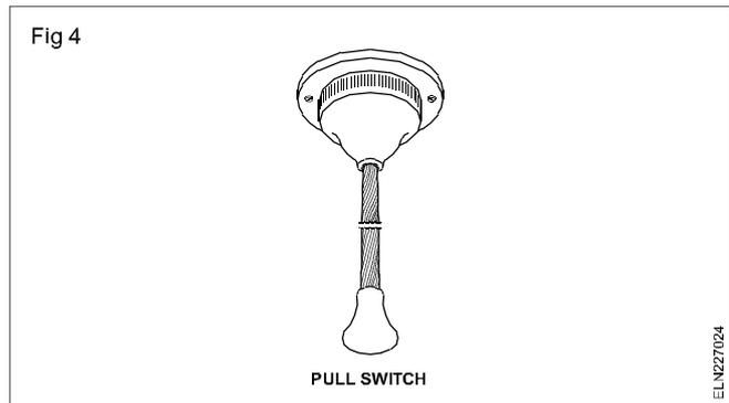
This switch is mounted on ceilings. As the user could operate the switch from a distance through the insulated cord, this could be used safely for operating water heaters in bathrooms or fan or lights in bedrooms.
