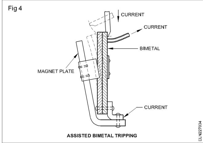
This method utilises the magnetic field which is produced when a current flows through the conductor. By locating the bimetal near to a substantial section of ferrous material, the magnetic field associated with current flowing in the bimetal will cause a sideways pull to be applied to the bimetal element, attracting the bimetal towards the ferrous material.
