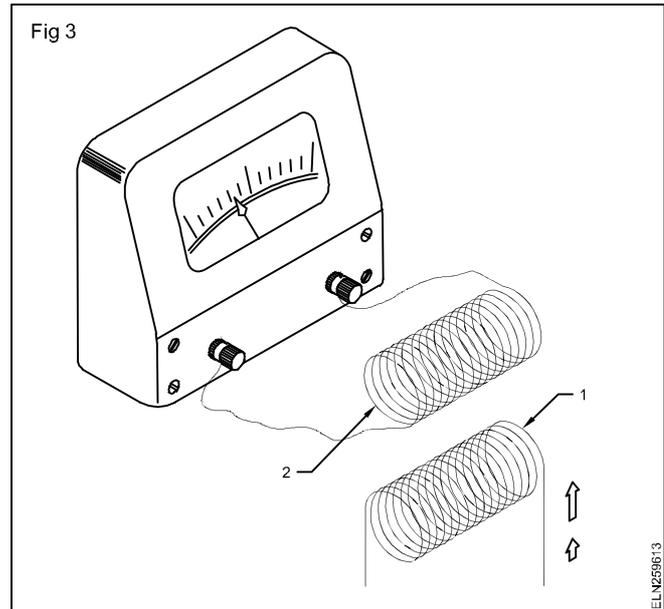
This induced emf will send the current, causing deflection of the meter. Introduction of a magnetic core between the coils increases the induced emf. The coil (1) is called primary and the coil (2) is called secondary.
