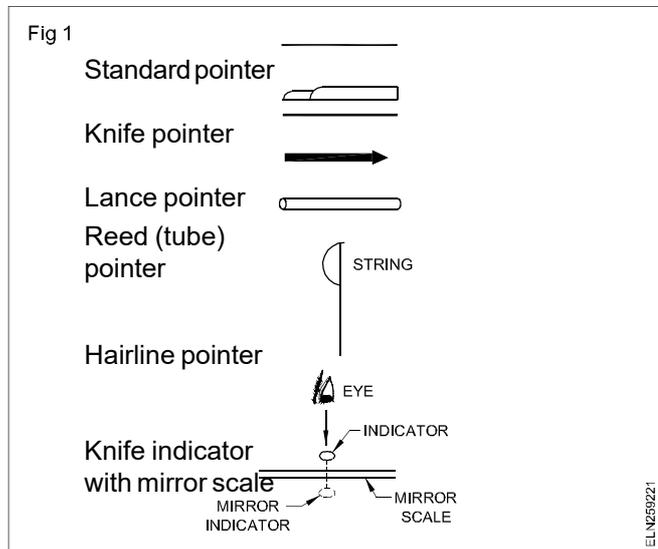
Due to the gap between the pointer and the scale, while reading an instrument, a slanting view may be obtained. Depending on the eye angle, a reading error may exist. This error is known as parallax error.
