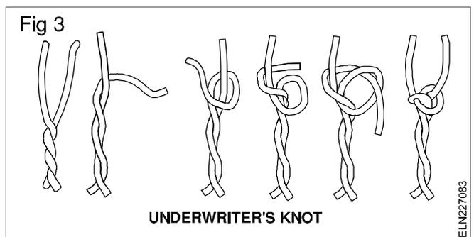
A knot is made on twin-twisted or twin-core flexible cable inside the accessories' cap cover.
