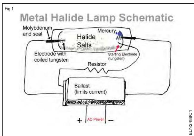
When the lamp is cold the halides and mercury are condensed on the fused quartz tube. When the lamp is turned on current passed through the starting electrode and jumps the short distance to the main electrode (Fig 1), this is aided by argon gas. The argon strikes an arc at low temperatures.
