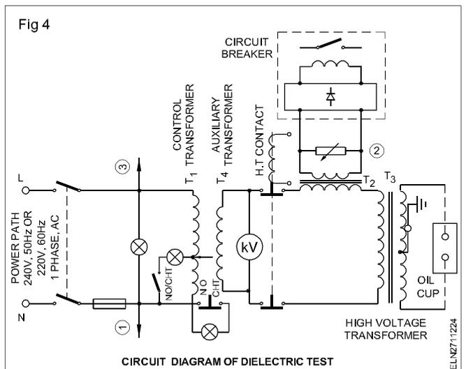
For conducting dielectric test on transformer oil, the oil is to be gently agitated and turned over several times so that homogeneous distribution of the impurities contained in the oil is spread all over.
