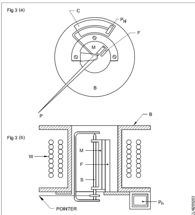
**Deflecting torque and graduation of scale:** However, in the moving-iron instruments, the deflecting torque is proportional to the square of the current passing through the coil. As such the scale of this instrument will be uneven. It is cramped at the beginning and open at the end (Fig 4).
