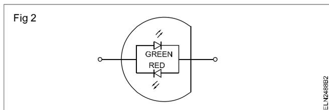
In a two-colour LED, two LEDs are connected in inverse parallel, so that one of the colour is emitted when the LED is biased in one direction and the other colour is emitted
