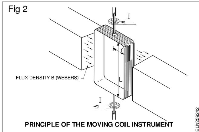
$I$  - The current in amperes passing through the coil and  $N$  is the number of turns.
