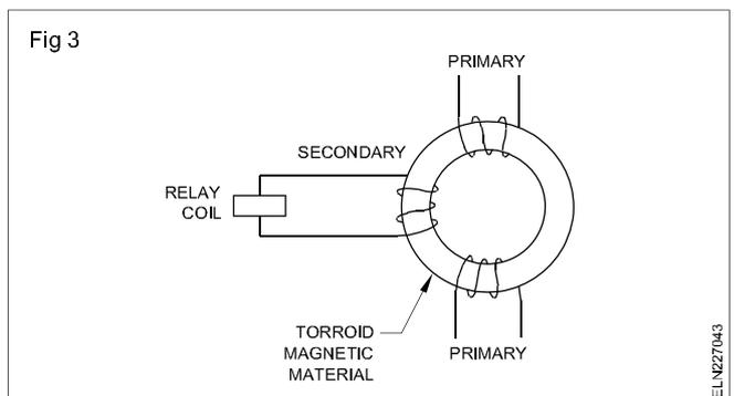
The main contacts are closed against the pressure of a spring which, provides the energy to open them when the device trips. Phase and neutral current pass through identical coils wound in opposing direction on a magnetic circuit, so that each coil will provide equal but opposing numbers of ampere turns when there is no residual current. The opposing ampere turns will cancel and no magnetic flux will be set up in the magnetic circuit.
