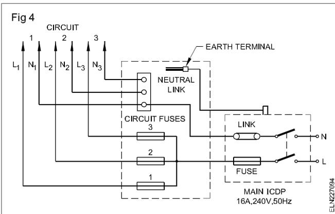
As each circuit can have power up to 800 watt, the phase wire which is taken from the circuit fuse of the distribution board is looped to the other light switches or fan switches of the same circuit by any one of the following ways.
