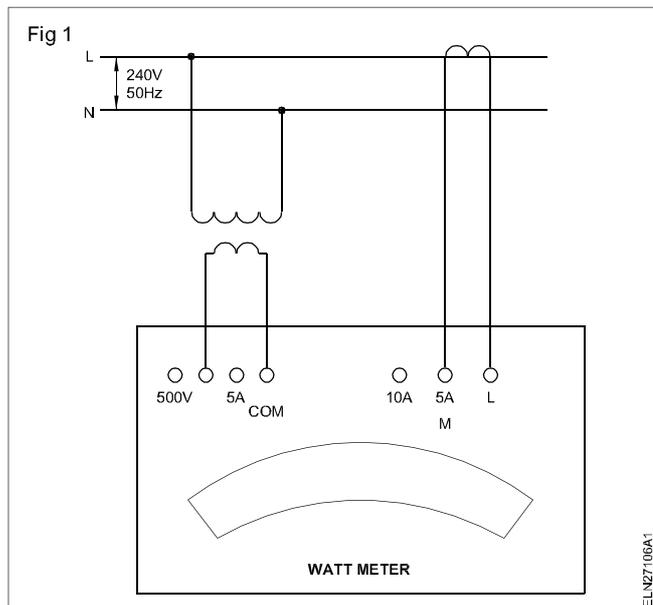
The maximum dial reading (Full scale deflection FSD) indicates 625 watts. Find the meter constant and actual power if the meter reads 600 watts against the following ranges.
