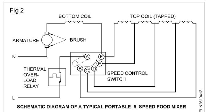
**Maintenance and servicing of a food mixer:** The manufacturer's service manual, if available, read it a number of times and follow the instruction. First listen to the complaint from the customer and make a note of it. Visually check the mixer right from the plug to the speed selector switch connections and enter the details in the maintenance card.
