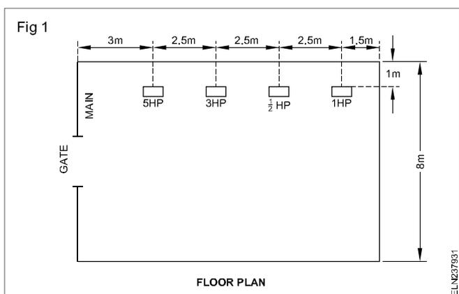
$$\text{FL current of 5HP motor} = \frac{5 \times 735.5}{\sqrt{3} \times 400 \times 0.85 \times 0.8} = 7.8A$$
