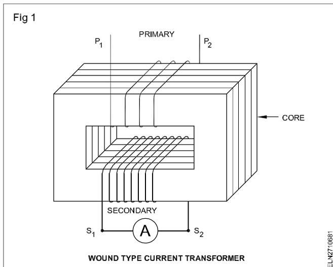
Fig 1 shows the connections of a wound type current transformer having a rectangular type of core. In general the ammeter is arranged to give full scale deflection with 5A or 1A when connected to the secondary of the current transformer.
