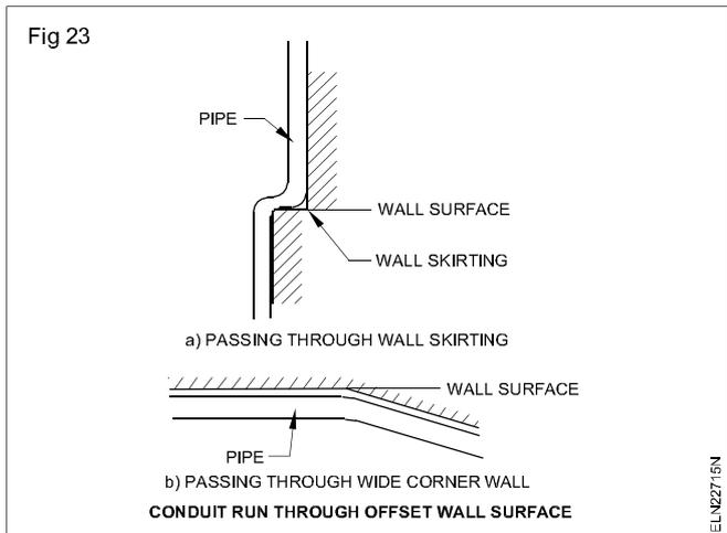
The bending may be done by using a simple bending block or by a hickey or with the help of a bending machine. Further, in concealed conduit wiring, the B.I.S. recommends bending of conduit pipes in preference to the use of bends and elbows.
