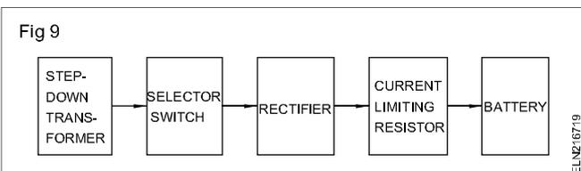
The transformers used for battery charging are generally provided with a number of tappings on their secondary side. In addition to stepping down the voltage, the transformer also serves another very important role. It isolates the charging circuit completely from the AC mains and thus completely eliminates the danger of electric shock from high voltage AC mains.
