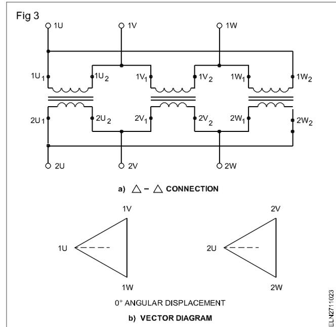
**Delta - Delta or  $\Delta/\Delta$  connection:** Fig 3 shows three transformers, connected in  $\Delta$  on both primary and secondary sides. There is no angular displacement between the primary and secondary line voltages. An added advantage of this connection is that if one transformer becomes disabled, the system can continue to operate in open-delta or in V-V. In V-V it can be operated with a reduced capacity of 58% and not 66.6% of the normal value.
