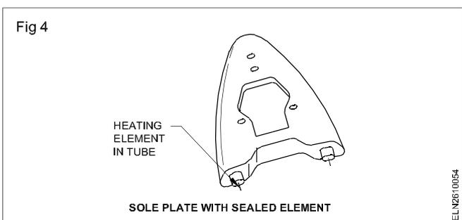
**Sole-plate:** The transfer of heat from the heating element within to the material being ironed is done by the sole-plate (Fig 4). The material being pressed can be easily damaged if the sole-plate is not smooth and free from scratches. If the sole-plates are scratched, they can be buffed and polished.
