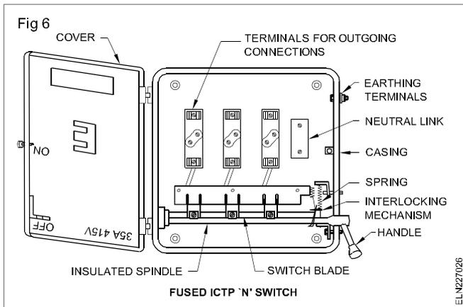
These switches need to be earthed through an earth terminal or screw provided in the outer casing.
