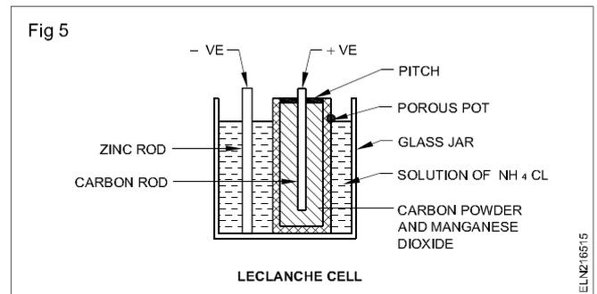
**Dry cell (Carbon-Zinc cell):** The danger of spilling the liquid electrolyte from a Leclanche type of cell led to the invention of another class of cells called dry cells.
