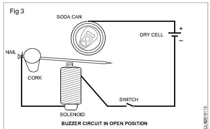
Then the circuit completes the current flow again and repeats the cycle. Each time the nail strikes back at the can, a sound is produced. Depending on the distance between the electromagnet and the nail several sound is produced.
