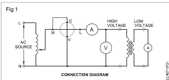
The low voltage side of the transformer is short circuited. A reduced voltage applied on the high voltage winding of the transformer such that the rated current flows through the ammeter. In this condition the impedance of the transformer is merely as equivalent impedance (Fig 2).
