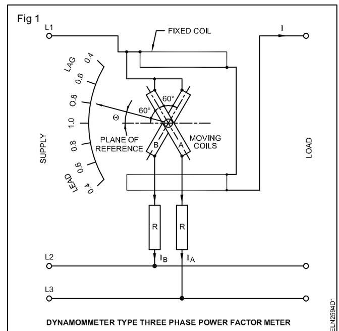
In this meter, the field coils are connected in series with the load along with one phase. The two moving coils are rigidly attached to each other at an angle of  $120^\circ$ . These coils are connected to two different phases. A resistance is connected in series with each coil.
