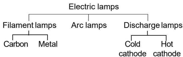
**Filament lamp:** A lamp in which a metal, carbon or other filament is rendered incandescent by the passage of electric current.
