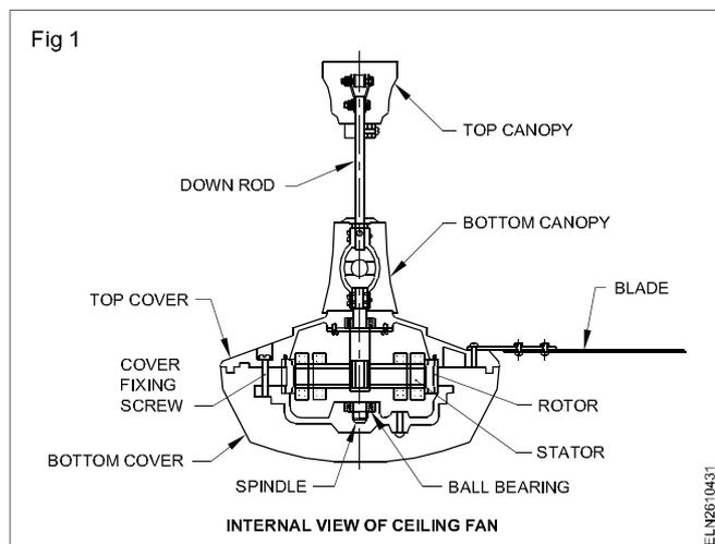
The rotor and the bottom cover are integrally diecast in high conductivity aluminium alloy which gives better accuracy and thus improves the efficiency of the cooling system.
