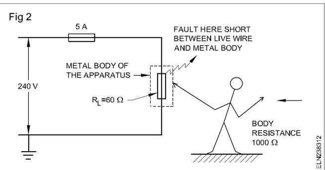
The value of current through the body =  $\frac{V}{R_{\text{Body}}}$
