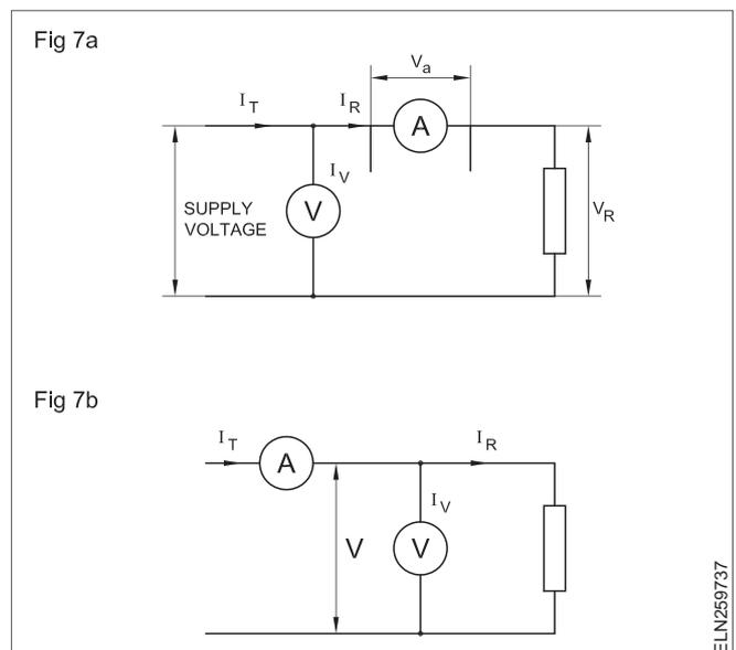
In both the cases, if readings of the ammeter and voltmeter are taken, then the measured value of resistance is given by
