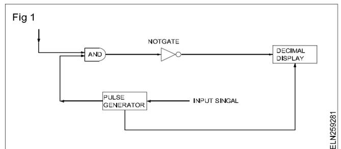
**Input signal:** It is basically the signal of voltage to be measured.
