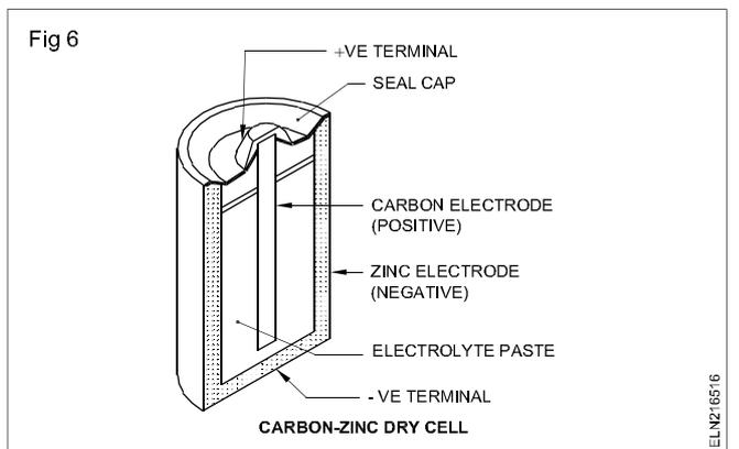
As with all primary cells, one of the electrodes becomes decomposed as part of the chemical reaction. In this cell the negative zinc container electrode is the one that is used up. As a result, cells left in equipment for long periods of time can rupture, spilling the electrolyte and causing damage to the neighbouring parts.
