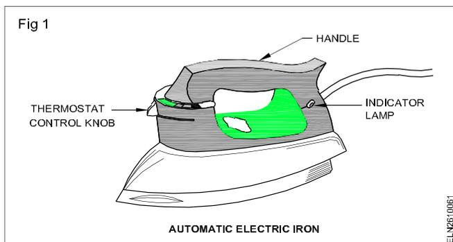
Automatic irons are fitted with a thermostatic switch to regulate the heat to a specific predetermined value. The thermostatic switch disconnects the supply when the predetermined value is reached and reconnects the supply when the iron cools down. A turning knob with a dial just below the handle, marked as rayon, cotton, silk, wool etc. can be operated to select the preset temperature.
