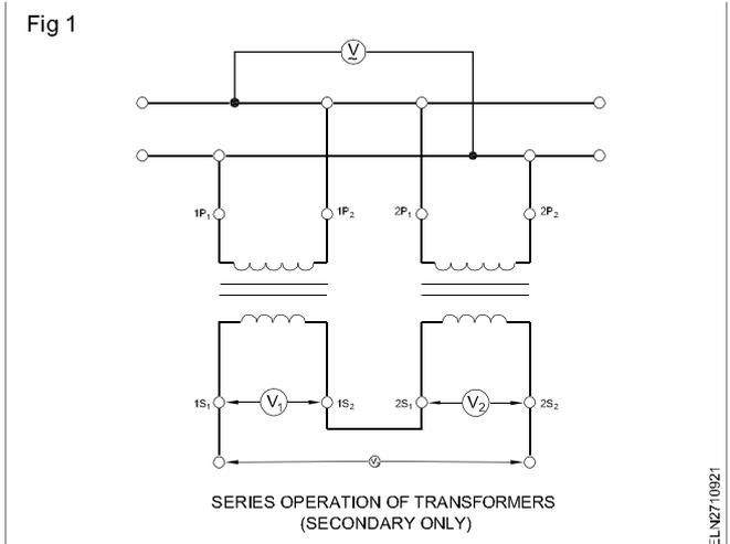
In series operation, individual secondary voltages of both transformers are added if they are connected with proper polarity, but the current ratings are remains same.
