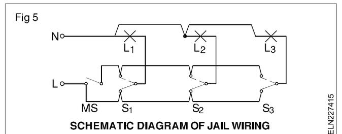
The master switch (MS) could be operated by the warden to make all the lights ON when they are all OFF.
