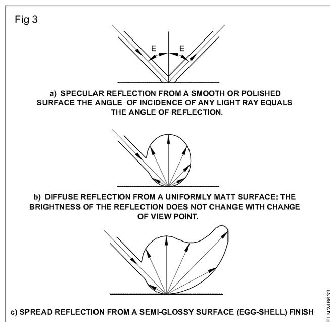
**Specular reflection:** When light strikes a mirror like surface it is reflected at the same angle and in the same plane as it strikes, for example a car lamp.
