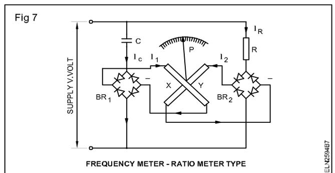
**Working:** The current through the coil depends upon the supply frequency. At higher frequency, the current through the coil X is higher whereas the current through coil 'Y' is independent of the frequency. The torque developed in the coil depends upon the interaction between the permanent magnetic field and the resultant field created by the coil currents.
