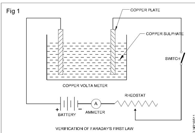
The negative electrode is dried and weighed. After passing a definite amount of current (which can be adjusted by the rheostat) for a definite time, the cathode is weighed again, after being dried once again.
