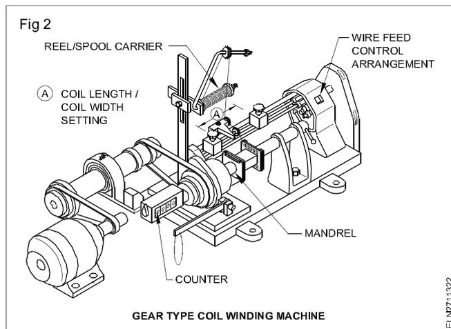
**Coil length setting or layer width setting:** To wind the coil of a designated length i.e. within the inner length of the bobbin two latches are provided on the transverse pulley mechanism to stop and reverse the feed at the desired point (Fig 3).
