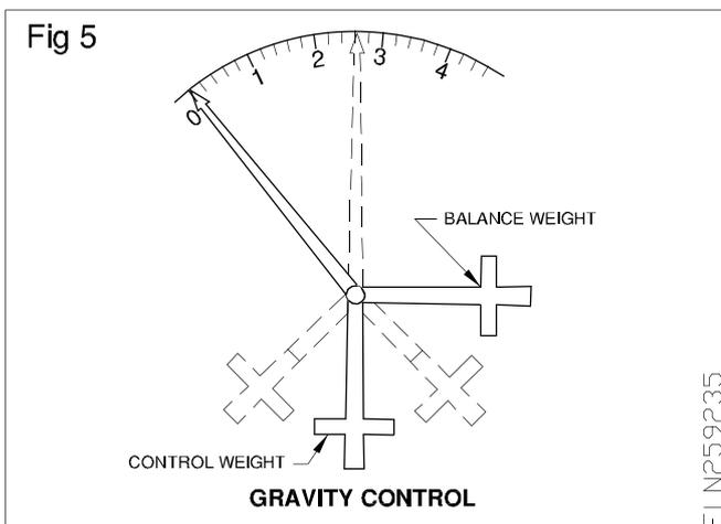
When the instrument is not connected to the supply, the control weight and the balance weight attached to the opposite end of the pointer make the pointer to be at zero position (Fig 5). When the instrument is connected to the supply, the pointer moves in a clockwise direction, thereby displacing the weights (Fig 5). Due to the gravitational pull, the weights will try to come to their original vertical position, thereby exerting a controlling force on the movement of the moving system.
