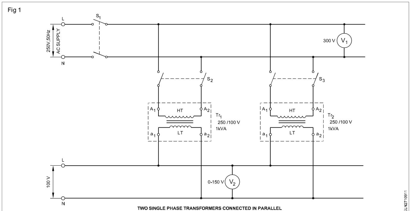
**Voltage ratio:** If voltage readings on the open secondaries of various transformers, to be run in parallel, do not show identical values, there will be circulating currents between the secondaries (and therefore between primaries also) when the secondary terminals are connected in parallel. The impedances of transformers is small, so that a small percentage voltage difference may be sufficient to circulate considerable current and cause additional  $I^2R$  loss.
