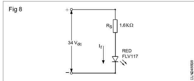
Note that, the maximum reverse voltage that can be applied for the chosen LED is only 8 volts. If accidentally a reverse voltage greater than 8 volts is applied, the LED will get damaged permanently. One way to protect the LED is by connecting a rectifier diode in parallel to the LED Fig 9.
