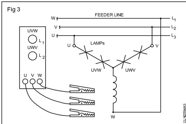
**Phase-sequence indicator using capacitor & lamps:**
