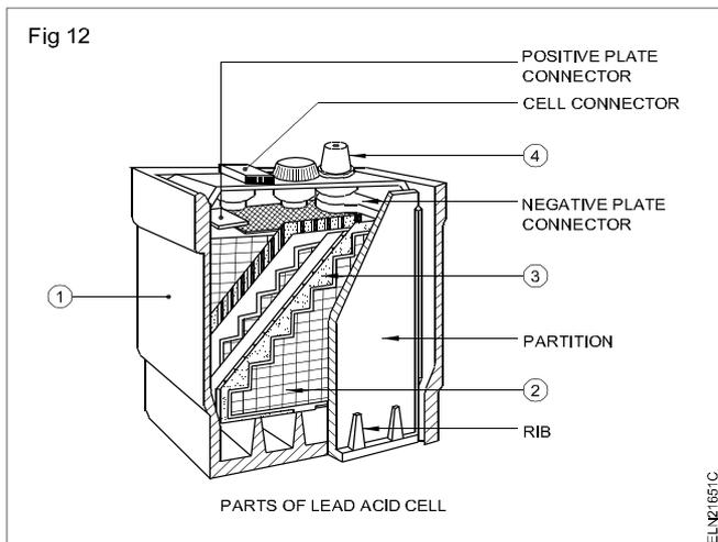
**Plates:** Positive plates are of two types.
