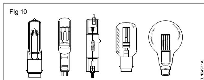
Most quartz lamps last as long as 250 hours and have a colour temperature rating of 3,200°K. Outputs vary from 150 to 350 watts for battery lights and from 200 to 10,000 watts for main power supply use. The quartz bulb itself
