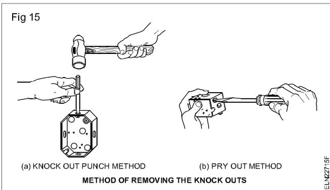
After removing the knock-outs, the conduit is to be fitted in the opening by any one of the methods shown in Fig 16.
