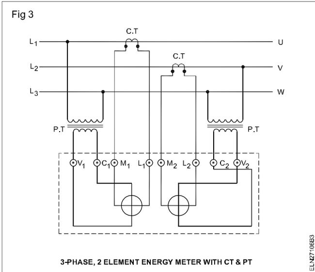
The metering cubicle used along with HT line of 11kV or higher voltages consists of 2 or 3 CTs and a three phase PTs known as a kiosk.
