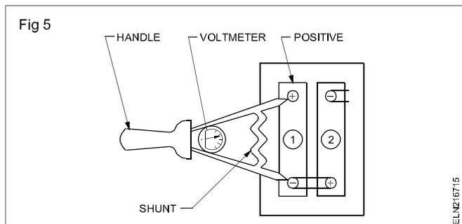
**Voltage of each cell:** The voltage of the cell is measured with a M C voltmeter. The fully charged cell will indicate 2.5 to 2.6V and a fully discharged cell will indicate 1.8V to 1.6V.
