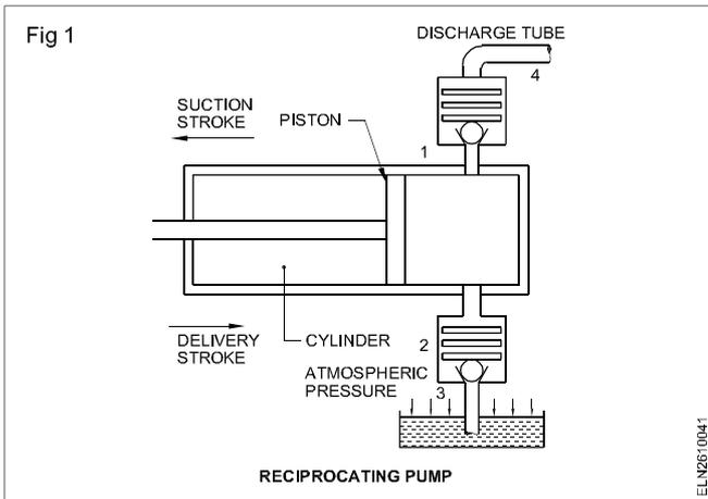
2 Fig 1 opens and allows the water to fill the cylinder through the suction pipe 3 due to atmospheric pressure outside. This stroke of the piston is called suction stroke.
