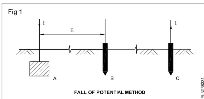
An alternating current of  $I_{\text{amps}}$  magnitude is passed through the electrode A to the electrode C via the earth and the potential across electrodes A and B is measured.
