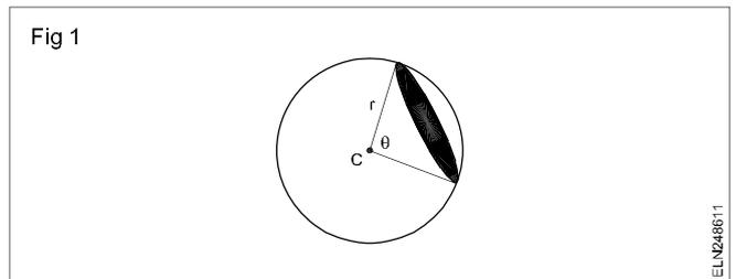
If the shaded area =  $r^2$  and a source of one candela is at the centre C, the light contained within the solid angle is one lumen.
