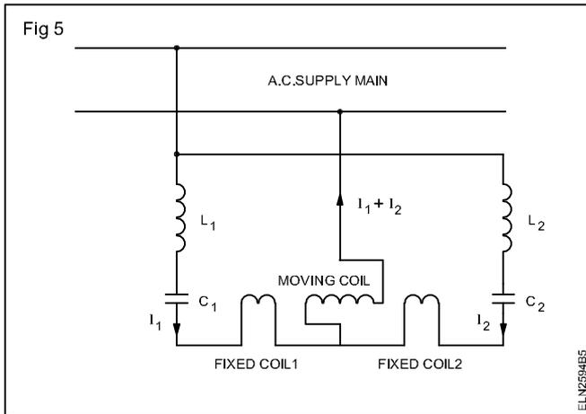
The resonant circuit of the fixed coil (1) is tuned for a frequency  $f_1$  and say 45 Hz, which is lower than the tuned frequency  $f_2$ , say, 60Hz of the fixed coil 2. The moving coil carries the vector sum of current  $I_1$  and  $I_2$  of the two fixed coils.
