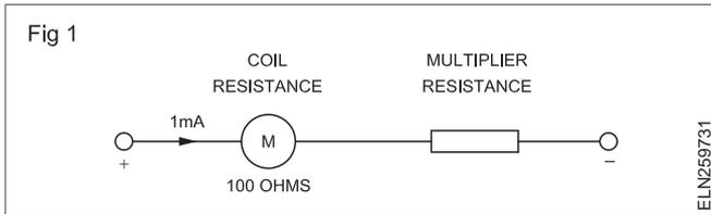
As such the total resistance between the terminals of the 10V voltmeter should be
