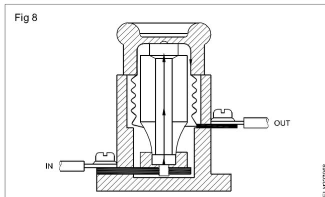
Diazed type fuses are available in two categories, a) quick-response type and b) delayed-action type. The quick-response type is used for heating circuits and normal loads whereas the delayed- action type is used for motor circuits and highly inductive circuits.
