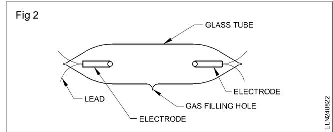
The length of the tube varies from 1 metre to 5 metres, and the diameter varies from 10 mm to 20 mm. The tubes are joined with electrodes which are operated at high voltage. The electrodes are connected with nickel wires for more length or to different letters. (Fig 3)
