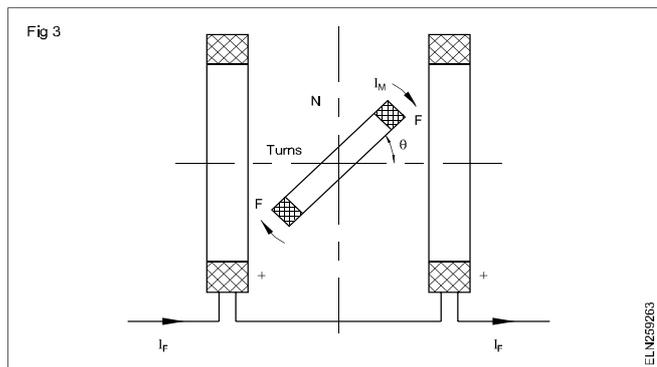
The deflecting torque is produced due to the interactions of the magnetic fields produced by the fixed and moving coils and will be proportional to the current carried by them.
