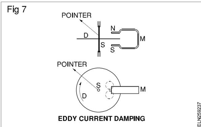
In the case of moving coil instruments, the moving coil is wound on a thin aluminium former. The eddy currents induced in the former produces the damping force.
