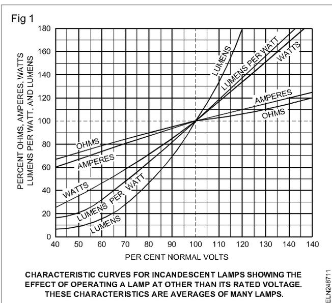
**Calculating the hot resistance:** The lamp filament operates at a very high temperature, 1800°C to 2200°C. Therefore, there is a very big difference between 'cold
