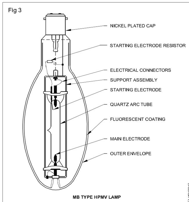
The wattages available are 80 watts 125 W, 250 W, 400 W, 700 W and 1000 watts operating in 230V/250V, 50 Hz main supply.
