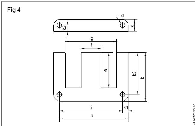
The nearest size sheet should be selected from the standard size of the stamping table. Here we assume the centre limb width to be 20 mm, and hence, the core E.I. 60 is selected. However, you may select any other type to suit the cross-section. But the other details like the number of stampings and the bobbin dimensions may change accordingly.
