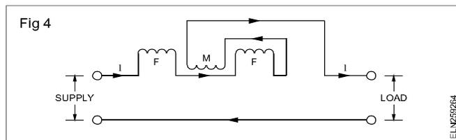
As the moving coil is made by winding small gauge (thin) wire, the above connection is unsuitable for measuring heavy currents.
