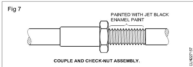
The exposed threaded portion of the long threaded conduit is painted with jet black enamel paint to prevent rust.
