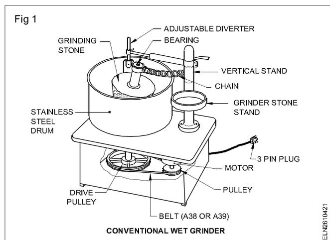
**Motor:** The motor used in the wet grinders is usually the capacitor start-induction motor (Fig 2 & 3). It has two windings. Both the starting and running windings are energised to start the motor, when the 70 to 80 % of the rated speed is reached, the starting winding is switched off by the centrifugal switching system. The motor then operates only on running winding.
