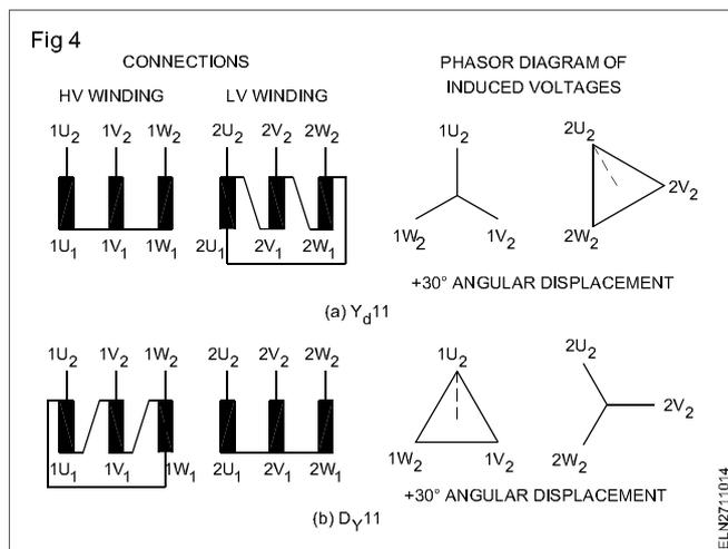
**Representation of phase displacement by hour hand of a clock:** The phase difference between the HV and LV windings for different types of connections can be represented by comparing it with the hour hand of a clock.
