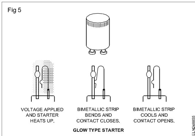
**Thermal type starter:** The switch has a bimetallic strip close to the resistance R which produces heat.
