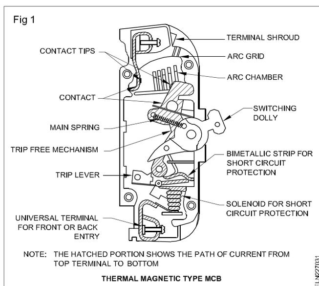
The electric current gets through two contact tips one each on moving and fixed contact of silver graphite.
