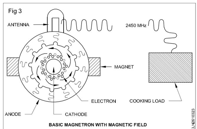
As the electrons approach the anode, they travel past the small resonant cavities to oscillate at a very high frequency of 2450 MHz. This RF energy is radiated into the cooking cavity where food is placed to be heated.
