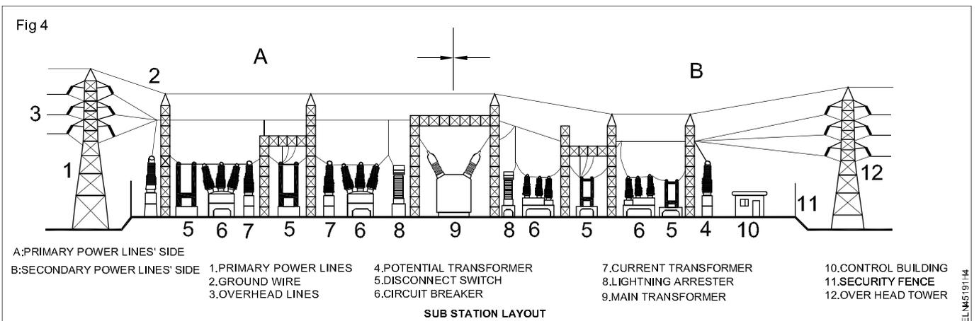
**Draw actual circuit diagram of substation visited and indicate various components**
