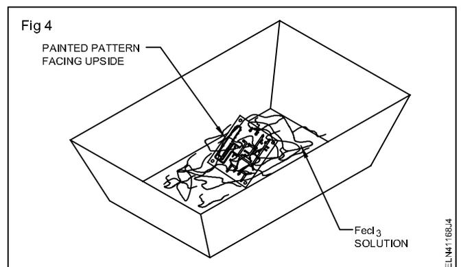
**Do not agitate the solution very fast as this may sometimes peel off the paint and etch the required patterns also.**
