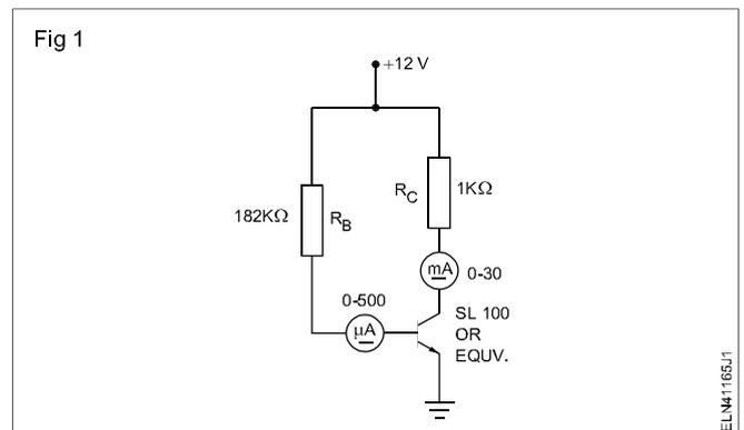
**The transistor is heated to observe the effect of heat on the set Q point of the transistor.**
