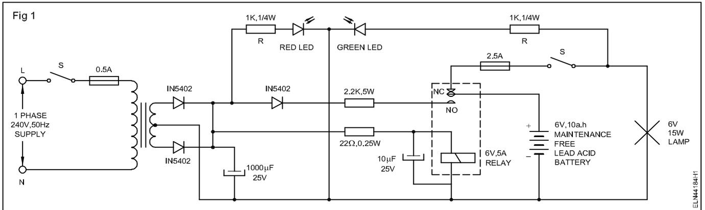
**TASK 2 : Construct inverter circuit for emergency light**
