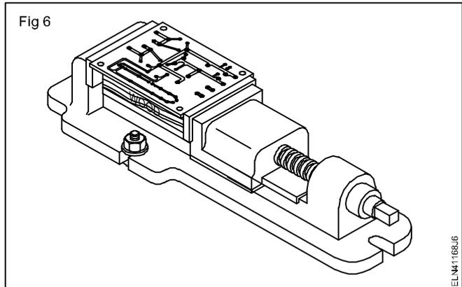
**Drill slowly and steadily. Careless drilling may pull the complete circular copper pattern away.**
