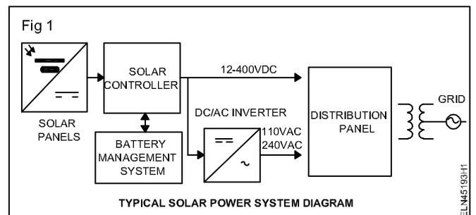
**Fig 1 is the model schematic diagram of solar power plant given for the general guidance of trainees. The trainees have to prepare and draw the schematic diagram of the solar power plant they visited.**
