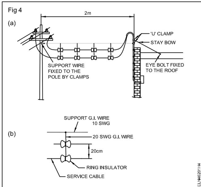
**Keep 20 cm gap between the ring insulators for 250 volt and 30cm for 440 volt.**
