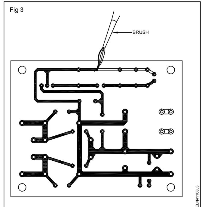
**If the ink flows slightly beyond the traced pattern circles and lines, do not try to correct it.**
