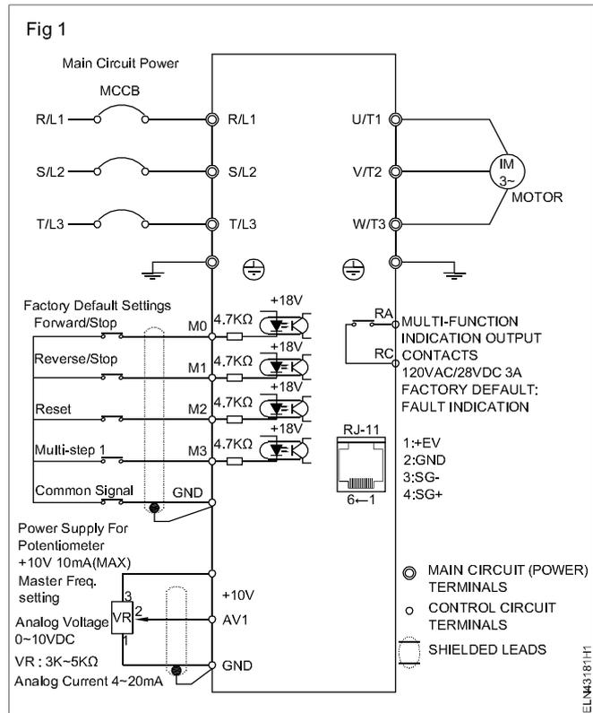
**TASK 3 : Reverse the direction of rotation in AC motor by setting in AC drive**
