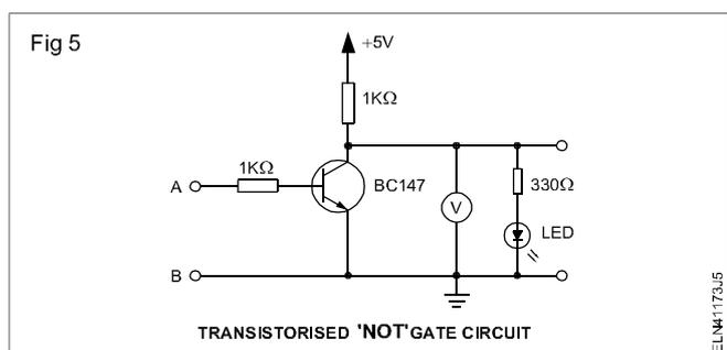
**When the input terminal of the circuit is grounded, it is equivalent to applying logic 0. Note that keeping input terminals open is not equal to logic 0 level.**
