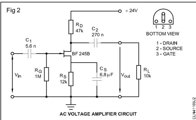
**Construct the circuit on a bread board or on a GPCB. If you are wiring the circuit on a GPCB use base for the FET to ensure that it does not get damaged.**
