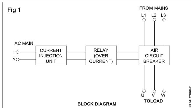
**Now the fault current set value is 2 Amp and the relay should trip in the time as per the dial indication.**
