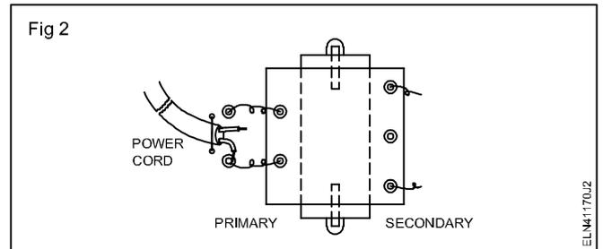
4 Using a continuity tester, check the power cord for any one of the following defects and record the defect observed if any;
