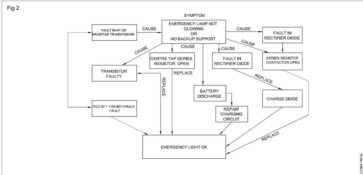
**TASK 3 : Test UPS and identify the faults and rectify**
