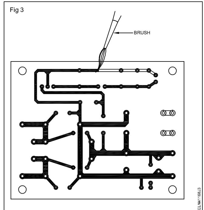
**If the ink flows slightly beyond the traced pattern circles and lines, do not try to correct it.**
