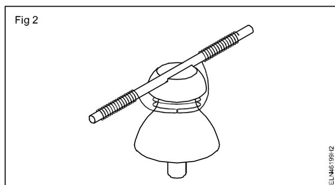
**Binding should be tighten without any gap. Where deviation or bend comes the ACSR conductor bind on the neck of the pin insulator. (Fig 3)**
