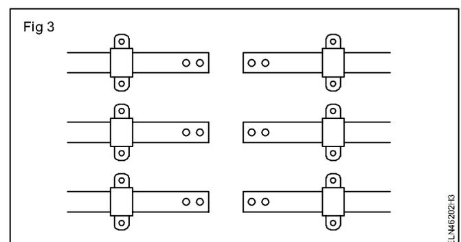
**If any over lapping ends of the busbar join by bolting together.**
