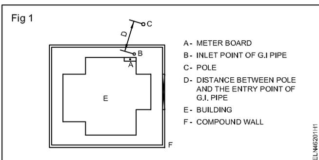
**Care should be taken to see that the service cable does not cross the adjacent building area. In some cases an intermediate pipe structure may be needed to avoid crossing.**
