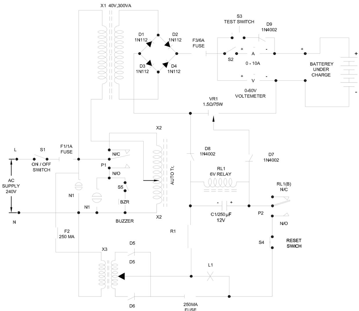
**The error indicator neon lamp (N2) and the buzzer stays on till the charger is reset.**
