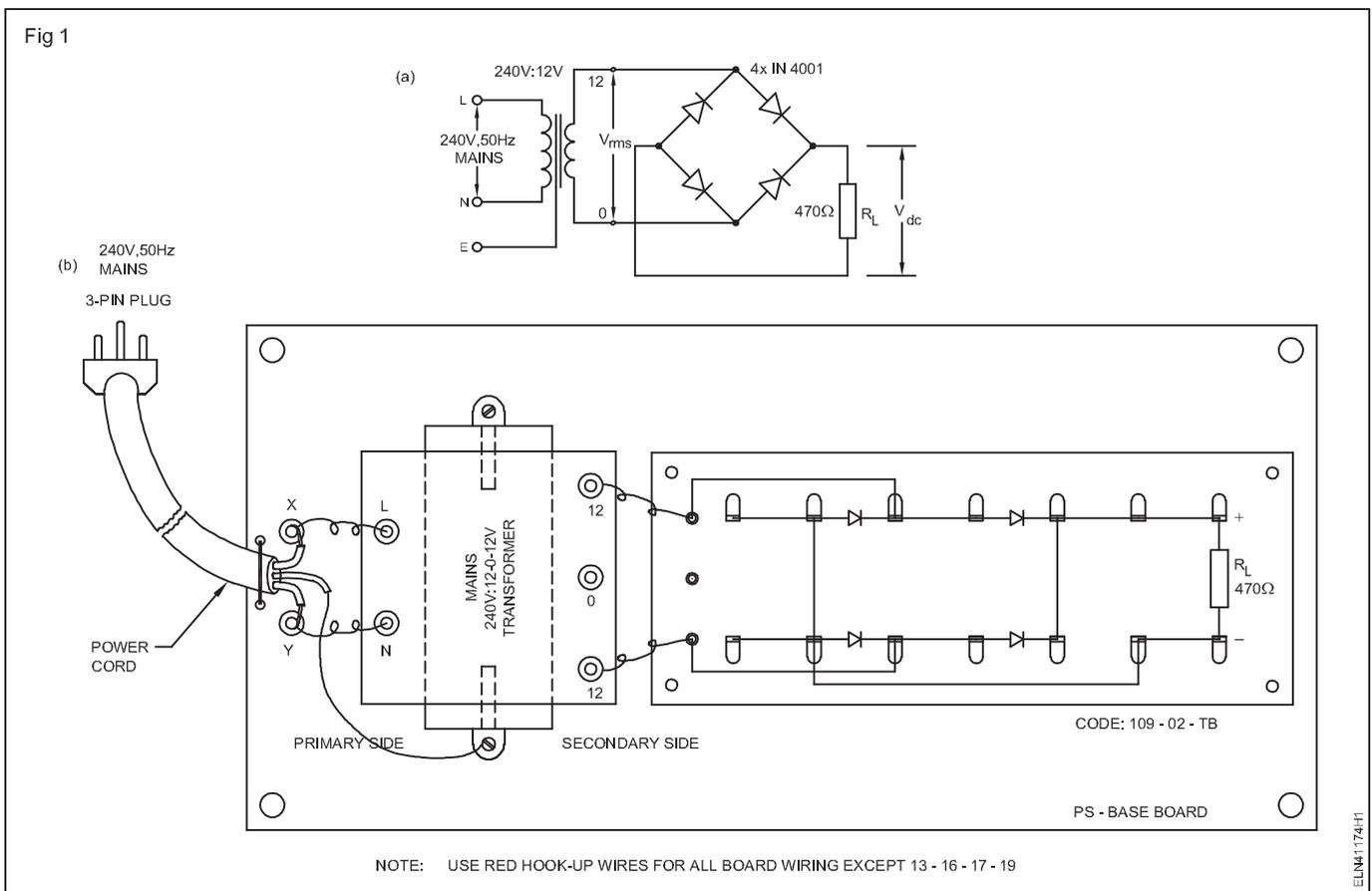
**TASK 2: Measure of ripple and calculate ripple factors in bridge rectifiers with RC filter**
