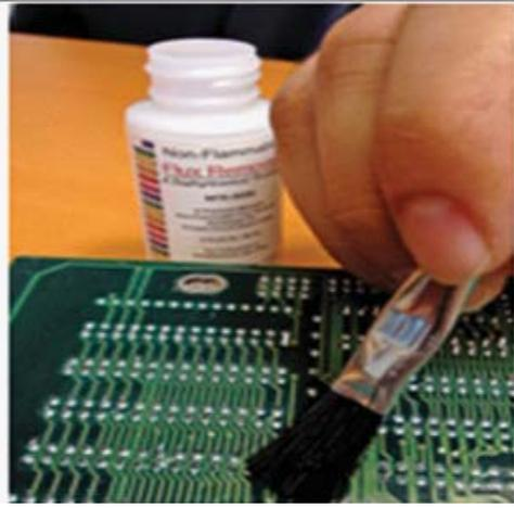
CLEANING PC BOARDS SOLDER JOINTS AFTER REWORK
