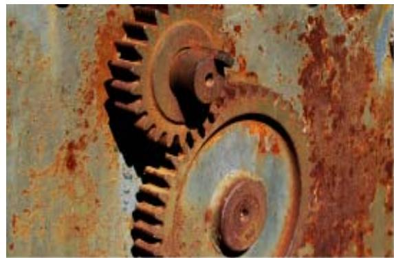
**Fig.2 Corroded gears**
