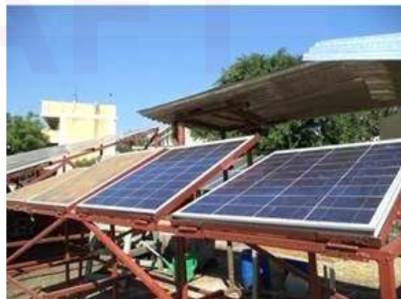
Fig. 1. Clean and dust PV module at 21.50 and 250 tilt angle.
