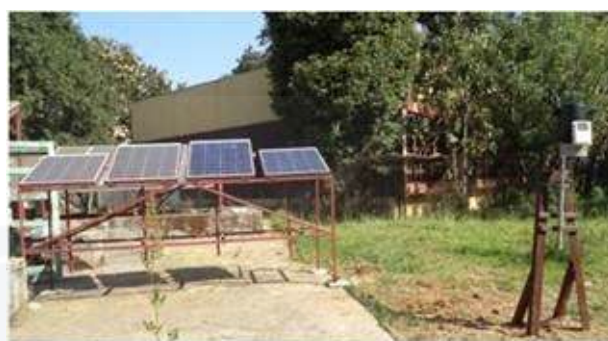
Fig. 3. Set up of vantage pro2 with clean and dusty PV module.
