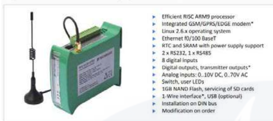
Programmable automation controller (PAC) with GPRS modem*
