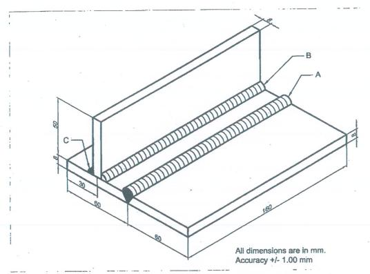
Weld by TIG welding Tee joint on aluminium sheets 3.15 mm thick as shown in figure given below. (100)
