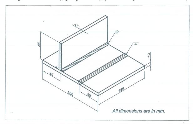
3. Job2. Weld by TIG welding aluminium sheets 2 mm thick as shown in figure given Below. (90)
